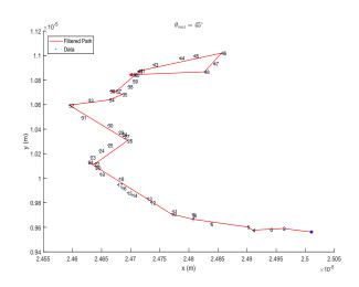
FIG. 6: The Cartesian position of a tracked particle path segmented using  $\theta_{\rm max} = 45^{\circ}$ . Blue dots with frame numbers mark the path. The red line indicates the new segmented path. The blue star marks the start position and the red star marks the end position.
