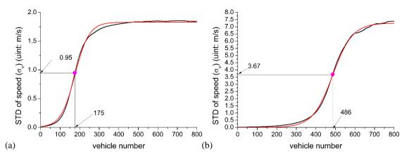
Fig. 3. The speed STDs of vehicles along a vehicle platoon. (a) the simulation results of the IDM and the speed of the leading vehicle is 10 km/h. (b) the simulation results of the FVDM and the speed of the leading vehicle is 60 km/h. The red dots are the transition points from convex to concave.
