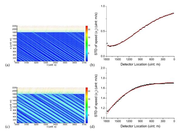
Fig. 2. Simulation results of the IDM. The parameters are set to:  $a_{max} = 0.73 \text{ m/s}^2$ ,  $b=1.67 \text{ m/s}^2$ , T=1.6 s,  $L_{veh} = 5 \text{ m}$ ,  $d_0 = 2.0 \text{ m}$ ,  $v_{max} = 80 \text{ km/h}$ ,  $d_r = 1 \text{ m/s}^2$ ,  $T_d = 2.5 \text{ s}$ ,  $x_0 = v_{last}T$ ,  $v_{new} = v_{last}$ . (a,c) The speed (unit: m/s) spatiotemporal diagram. (b,d) The STD of speed at each detector, in which the red line is the fitted curve. In (a,b),  $\gamma = 0.95$ ; in (c,d),
