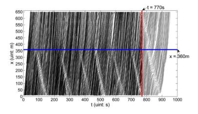
Fig. 8. The NGSIM trajectories on the leftmost lane collected during the time interval 07:50am-08:05am.
