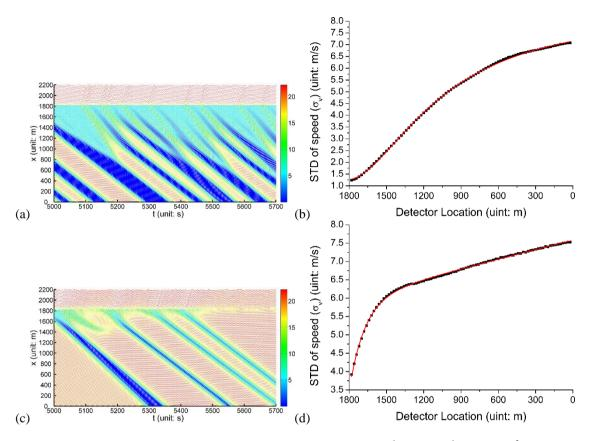
Fig. 4. Simulation results of the FVDM. The parameters are set to:  $\kappa = 0.2 \text{ s}^{-1}$ ,  $\lambda = 0.5 \text{ s}^{-1}$ ,  $d_r = 1 \text{ m/s}^2$ ,  $T_d = 2.5 \text{ s}$ ,  $x_0 = d$ ,  $v_{\text{new}} = V_{opt}(d)$ , d = 30 m. (a, c) The speed (unit: m/s) spatiotemporal diagram. (b, d) The STD of speed at each detector, in which the red line is the fitted curve. In (a, b),  $\gamma = 0.95$ ; in (c, d),  $\gamma = 0.5$ .
