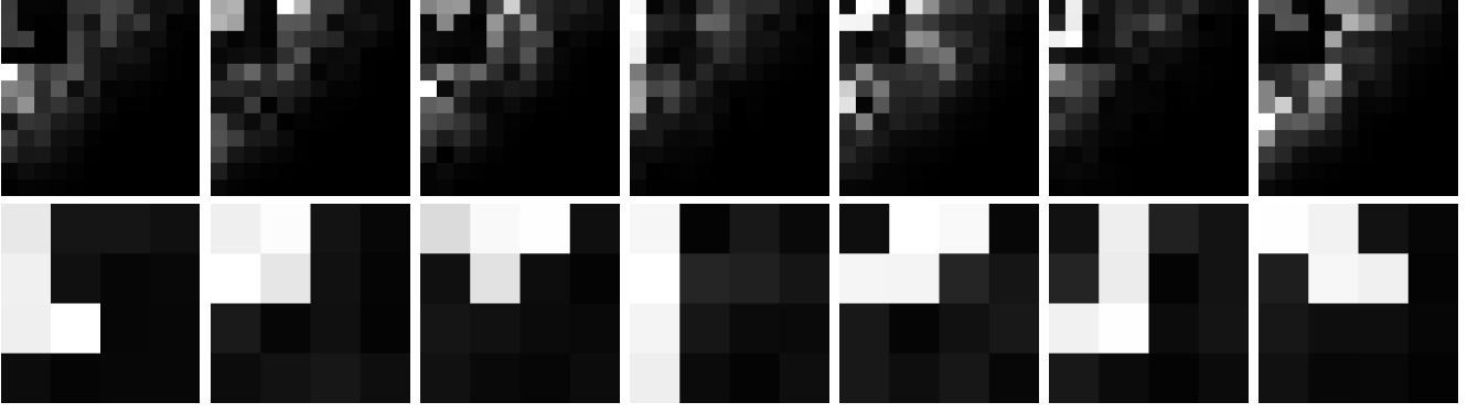
FIG. 10. Experiment C. Output images for the ‘LOTISJZ’ tetromino image data. The top row shows the output two-mode states where the intensity of the pixel in the i th row and j th column is proportional to the probability of finding i photons in the first mode and j photons in the second mode. The bottom row is a close-up in the image Hilbert space of up to 3 photons, renormalized with respect to the probability of projecting the state onto that subspace. In other words, this row illustrates the states |\psi_i\rangle of Eq. (44). The fidelities of the output states |\psi_i\rangle with respect to the desired image states are respectively 99.0%, 98.6%, 98.6%, 98.1%, 98.0%, 97.8%, and 98.8% for an average fidelity of 98.4%. The probabilities p_i of projecting the state onto the image space of at most three photons are respectively 5.8%, 36.0%, 21.7%, 62.1%, 40.7%, 71.3%, and 5.6% .
