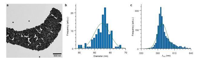
**Figure S1** | **Characterization of gold nanospheres. a**, Representative transmission electron microscopy image of the gold nanospheres used in this work. **b**, The diameter distribution of the nanospheres from 127 individual particle is  $62.5\pm2.5$  nm.**c**, The resonance wavelength distribution of 2000 individual nanoparticles is  $588\pm8$  nm.
