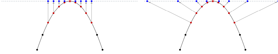
Figure 1. Projection of neighbouring points to the tangent space along the central normal (left), and the neighbour normals (right). The central point is shown with an additional circle around it, and all its neighbouring points are marked in red. The remaining black points on the manifold are shown for reference. The projected locations on the tangent space are marked in blue. The manifold is shown in black, while the tangent line at the central point is shown with a blue dashed line.
