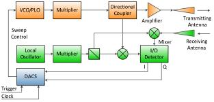
Fig. 1. Typical architecture of reflectometry
