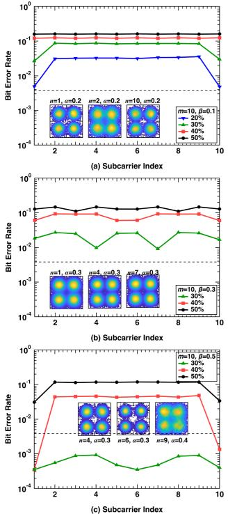
Fig. 3 BER plots for (a) m = 10 and  $\beta = 0.1$ , (b) m = 10 and  $\beta = 0.3$  and (c) m = 10 and  $\beta = 0.5$
