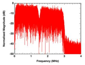
Fig. 5 The received electrical spectra of the 2-CAP signal showing the attenuation caused the low modulation bandwidth of the LED for  $\alpha = 0$  and  $\beta = 0.1$
