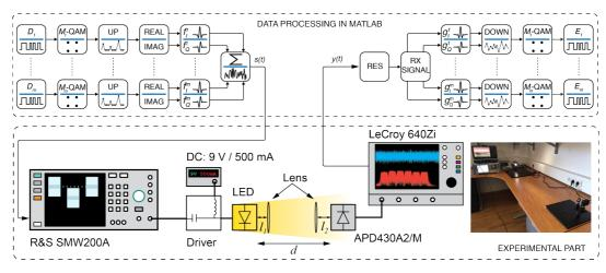
Fig. 1 The schematic block diagram of the experimental NM-CAP VLC system. 'UP', 'RES' and 'DOWN' blocks refer to up-sampling, resampling and down-sampling, respectively
