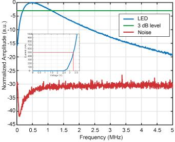
Fig. 2 The measured LED and noise frequency responses with the highlighted 3 dB level. The band-pass feature of the LED magnitude response is cause by the bias-tee acting as a high-pass filter and such, causing a cut-on effect at around 250 kHz. The measured cut-off frequency is around 1.25 MHz, giving an effective bandwidth of around 1 MHz. Inset, the measured I-V curve of the LED and drive circuit.
