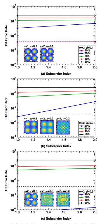
Fig. 4 BER plots for (a) m = 2 and  $\beta = 0.1$ , (b) m = 2 and  $\beta = 0.3$  and (c) m = 2 and  $\beta = 0.5$
