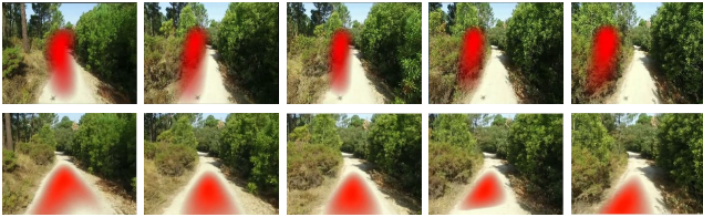
Fig. 16 Images of the result obtained by the original detector in a fault situation in the test performed on the complete video sequence of Video 12. In the first line is the result obtained by the original detector is shown, in the second line is shown the result obtained by the proposed system.
