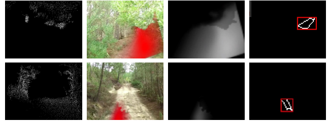
Fig. 19 Sub-set of typical results that demonstrate the operation of the Validator module. The first line illustrates the identification of a fault caused by the calculation of the optical flow. The second line illustrates the identification of a fault caused by an erroneous signaling of obstacles in the region where the path is located. The first column illustrates the projection of the obstacle presence information to the camera plane, the second column illustrates the result of the track detector, the third column illustrates the activity of the neuronal field, NF , and the fourth column illustrates the result obtained by the validator module.
