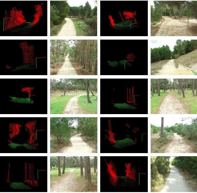
Fig. 13 Sub-set of typical results obtained with the set of test data, demonstrating the three-dimensional reconstruction of the environment described in front of the robot ( \approx 8\text{m} ). Images with three-dimensional reconstruction, first and third columns, illustrate the clouds of points obtained where, the red dots describe the obstacles and the green dots describe the ground plane.
