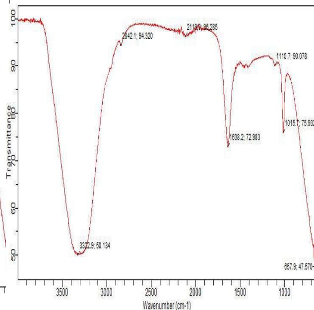
**Figure 4B:** A typical FTIR spectrum for Bauchi Liquid Harmattan Dust Sample
