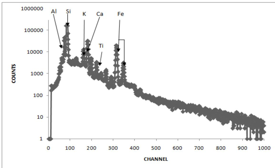
**Figure 6:** A PIXE Spectrum of Harmattan Dust Sample from Potiskum Deposit
