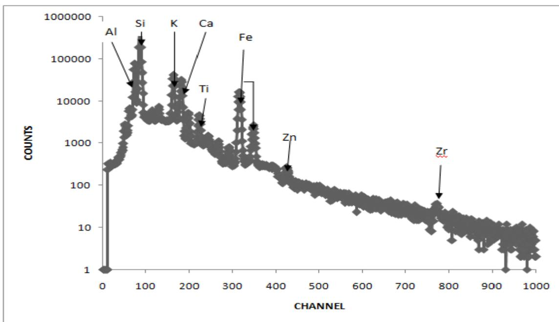
**Figure 5:** A PIXE Spectrum of Harmattan Dust Sample from Jos Deposit
