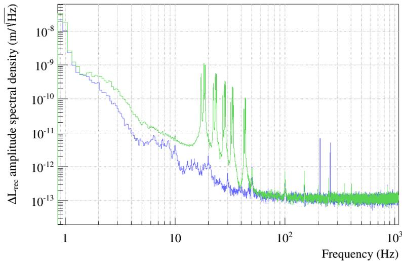
**Figure 2.** Amplitude spectral density of the reconstructed  $\Delta L$  signal in the free Michelson configuration. Two dataset are shown with different sinewaves excitations applied on the mirror actuators. Green: five sinewaves are applied between 15 Hz and 45 Hz to each of the three mirrors. Blue: two sinewaves are applied between 200 Hz and 250 Hz to each of the three mirrors. The plots are made from two dataset lasting for 60 s.
