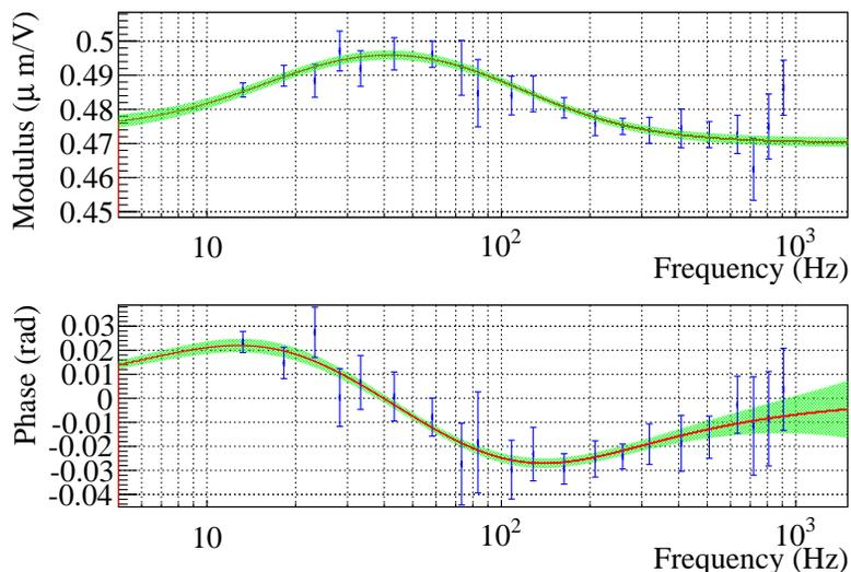
**Figure 3.** NE mirror actuator transfer function normalized by the mechanical transfer function and with the measured delay subtracted for a better visualization. Each blue point is an average over all the calibration measurements done at this frequency, with their  $1\sigma$  statistical uncertainty. The red line is the fitted model for the (normalized) actuator response. The green filled area represents the  $1\sigma$  statistical uncertainty as function of frequency.
