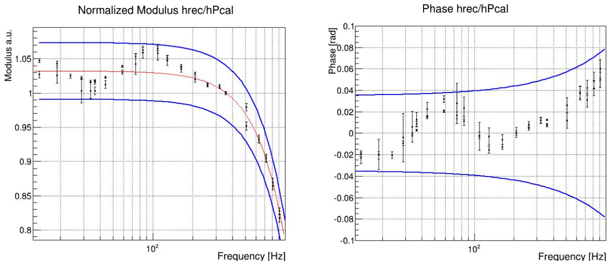
**Figure 6.** Left plot represents the normalized transfer function between the reconstructed lines amplitude and the PCal injected lines amplitude. The data points are fitted with a notch around 2 kHz and remain in the  $\pm 4\%$  error band. Right plot shows the phase of this transfer function with an error band of  $\pm 35 \pm 2\pi f \times 7e-3$  mrad.
