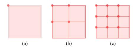
Fig. 2. Arrangements of displacement stacks of binary phase gratings for (a) original, (b) double, and (c) triple resolutions, which correspond to  $1^2$ ,  $2^2$ , and  $3^2$  displacement positions (red circles) within single grid (light-red square) of binary gratings, respectively.
