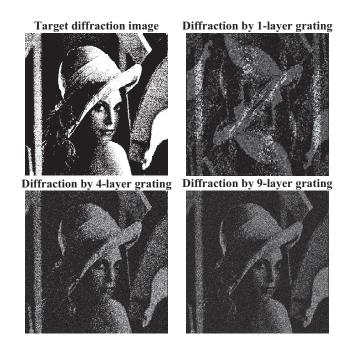
Fig. 3. Diffraction images of optical elements designed for different resolutions. (Upper left) Target of diffraction image, (upper right) diffraction image by single binary phase grating, (bottom left) double-resolution diffraction image by stacks of four binary phase gratings, and (bottom right) triple-resolution diffraction image by stacks of nine binary phase gratings.
