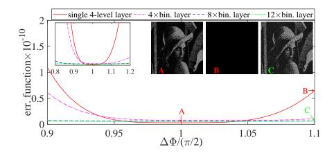
Fig. 4. Relations of diffraction deviations and incident wavelengths for (i) conventional 4-level phase grating, (ii) stacks of four binary phase gratings, (iii) stacks of eight binary phase gratings, and (iv) stacks of twelve binary phase gratings. The diffraction deviations are defined as an error function in the texts. The dependence of incidence wavelengths  $\lambda$  is related to the modulation phase  $\Delta \Phi \equiv \Delta n d / \lambda$  of the binary grating.
