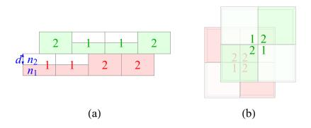
Fig. 1. Schematic diagram of displacement stacks of binary layers (a) in the side perspective and (b) in the top perspective, where displacement distance is set to be half of grid dimensions.
