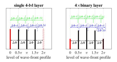
Fig. 6. Variations of histograms of wave-front profiles with respect to increasing and decreasing  $\Delta \Phi \rightarrow \Delta \Phi \pm \delta$  in (a) the conventional 4-level grating and (b) the 4×binary-layer optical element, as defined in Fig. 5(a-b).
