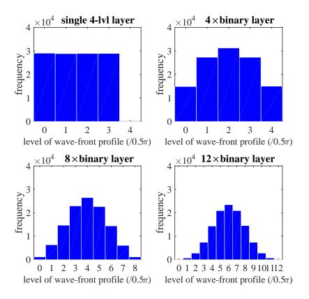
Fig. 5. Histogram of phase levels of wave-front profiles for optical elements using: (a) conventional 4-level phase grating, (b) displacement stacks of four binary gratings, (c) displacement stacks of eight binary gratings, and (d) displacement stacks of twelve binary gratings.
