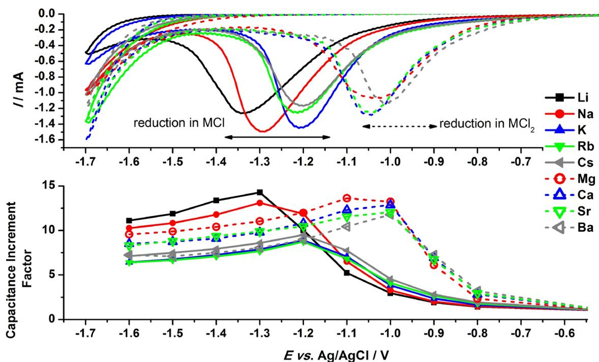
**Figure 2.** top panel: cyclic voltammograms of GO reduction in MCl and MCl<sub>2</sub> solutions (0.1 mol dm<sup>-3</sup>) (full lines – alkali metals, dashed lines – alkaline earth metals); bottom panel: capacitance increment factors as the function of reduction potential. GO films contained Vulcan XC-72R as conductive additive.
