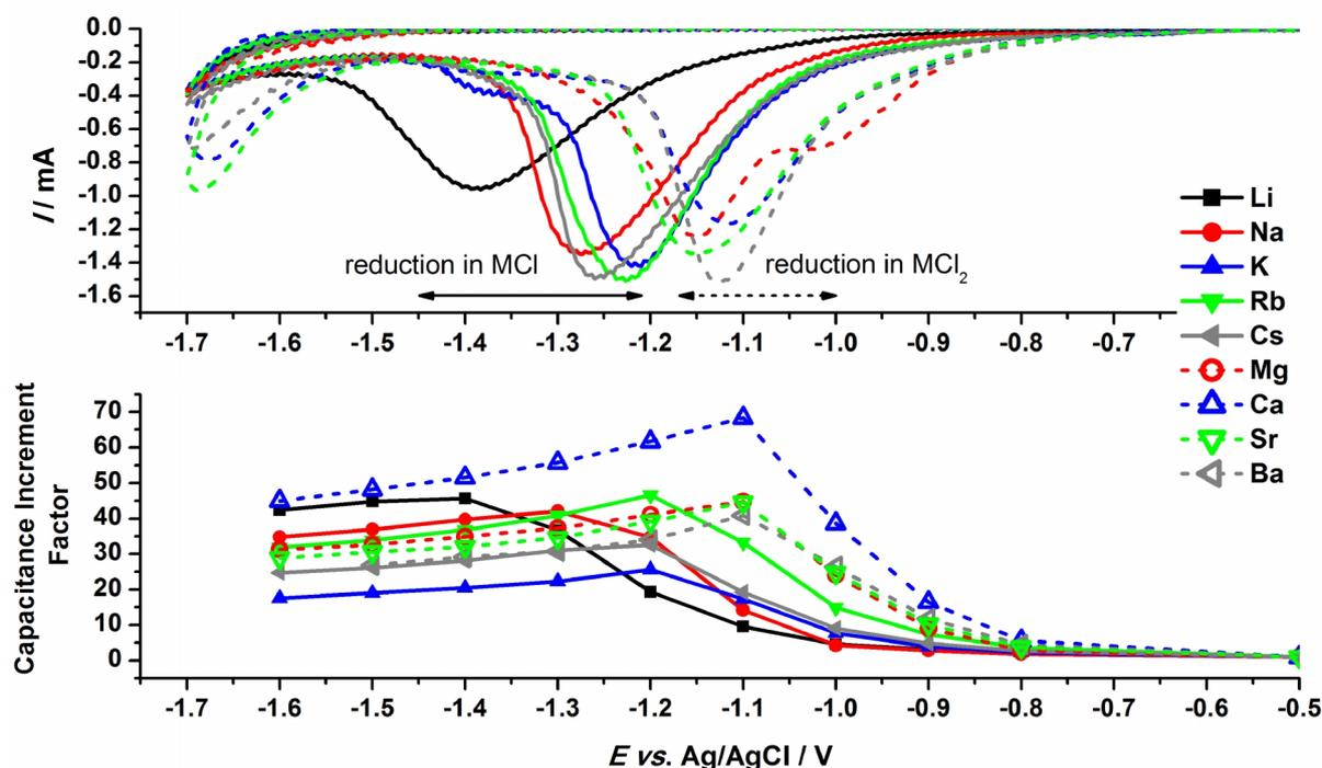
**Figure 1.** top panel: cyclic voltammograms of GO reduction in MCl and MCl<sub>2</sub> solutions (0.1 mol dm<sup>-3</sup>) (full lines – alkali metals, dashed lines – alkaline earth metals); bottom panel: capacitance increment factors as the function of reduction potential. For the presented measurements no conductive additive is used.
