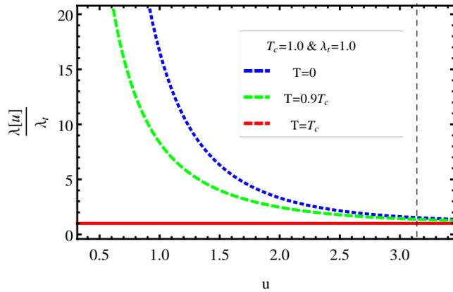
FIG. 2. Plots of normalized  $\lambda$  vs  $u$  given in (11) for  $T = 0.0$  (blue dotted line),  $0.9T_c$  (green dashed line), and  $T_c$  (red solid line). Here  $\lambda_t = 1.0$  and  $T_c = 1.0$ . The vertical dashed line indicates the position of  $\Lambda_{\text{QCD}} = \pi$ .
