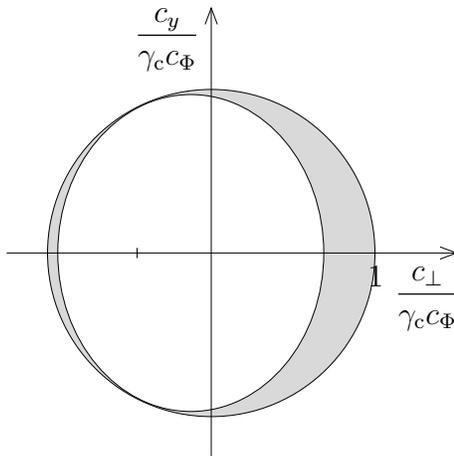
Figure 2: The points  $(\frac{c_\perp}{\gamma_c c_\Phi}, \frac{c_y}{\gamma_c c_\Phi})$  of the disk of radius 1 that yield QNSRs  $a \rightarrow \infty$  and  $a \rightarrow 0$  sit in the left and right shaded crescents, respectively.
