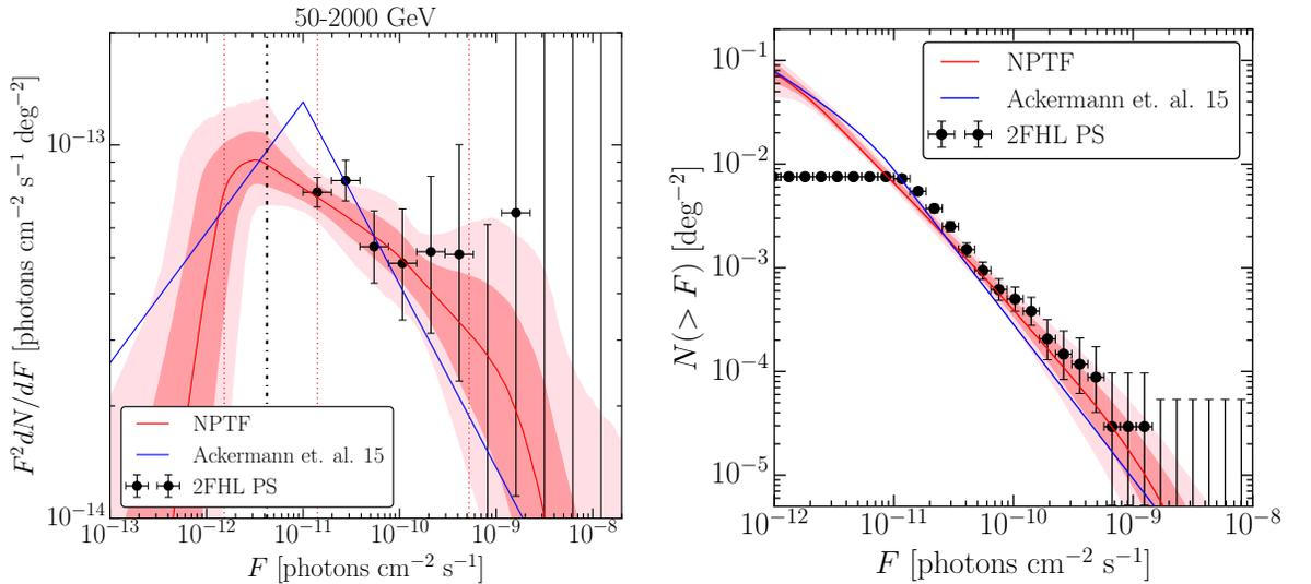
Figure 3.10: **(Left)** Best-fit source-count distribution in the wide-energy bin from 50–2000 GeV using all quartiles of Pass 8 *ultracleanveto* data. The black points indicate the 2FHL sources, and the blue line denotes the best-fit source-count from [163] that corresponds to the same energy bin. **(Right)** A comparison of the cumulative source-count distribution for the same analysis.
