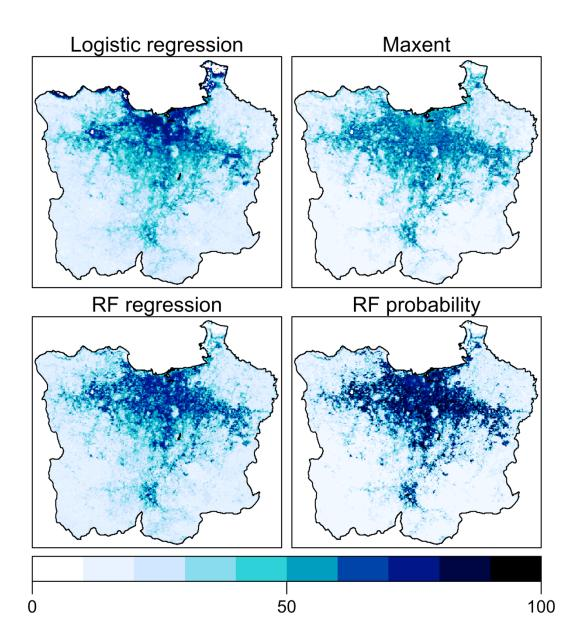
Figure 2. Predicted fractional impervious surface area (%) by four models for study 1: Logistic regression (Left upper), MaxEnt (Right upper), RF regression (Left bottom), and RF probability (Right bottom).
