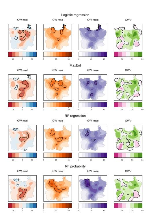
Figure 5. Spatial distributions of GW msd, GW mae, GW rmse, and GW r for fractional impervious surface area predicted from logistic regression, MaxEnt, RF regression, and class probability of RF classifiers for study 1. Black polygons represent 'significant' (p-values less than 0.01) areas by the Monte Carlo permutation tests.
