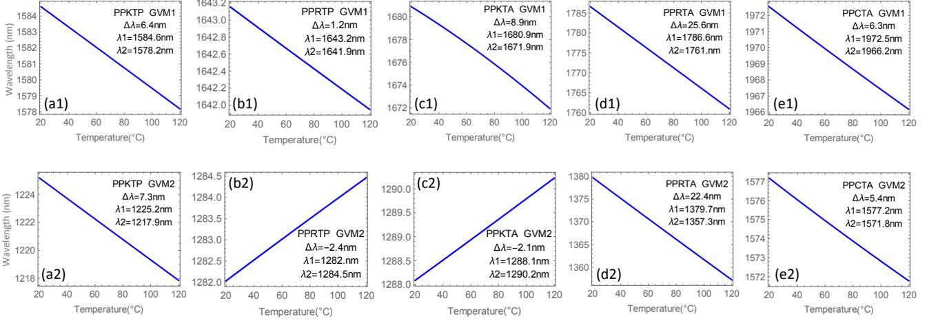
FIG. 1.  $\lambda_{GVM1}$  (first row) and  $\lambda_{GVM2}$  (second row) as a function of the temperature for different crystals. (a) PPKTP, (b) PPRTP, (c) PPKTA, (d) PRRTA and (e) PPCTA. Inset:  $\lambda_{1(2)}$  is the wavelength at 20 (120) °C, and  $\Delta\lambda = \lambda_1 - \lambda_2$ .
