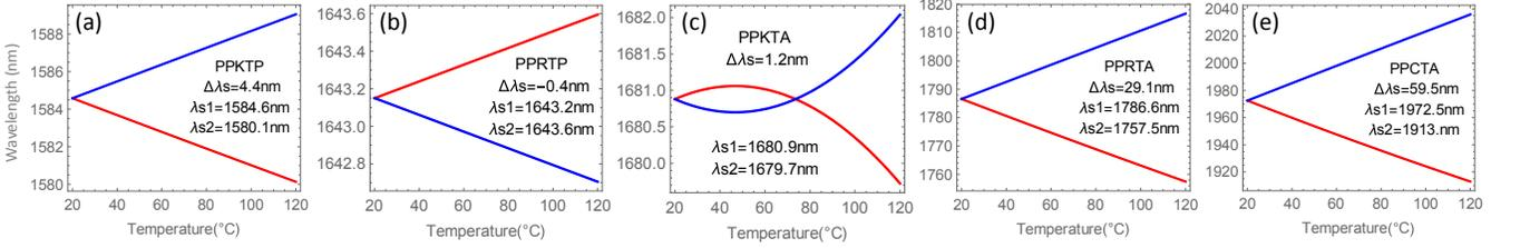
FIG. 2. The phase matched wavelength of signal (red line) and idler (blue line) as a function of temperature. (a) PPKTP, (b) PPRTP, (c) PPKTA, (d) PRRTA and (e) PPCTA. Inset:  $\lambda_{s(2)}$  is the wavelength of the signal at 20 (120) °C, and  $\Delta\lambda_s = \lambda_{s1} - \lambda_{s2}$ . In these plots, the poling period for each crystal is fixed to satisfy the degenerate type-II GVM1 condition at 20 °C.
