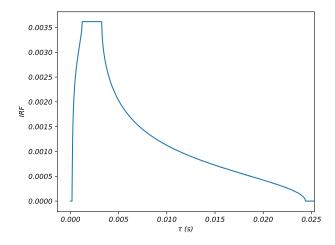
**Figure 5.** Impulse response function of the disc required for fit of Fig. 4, inferred from parameter  $r_o$  and equation (8).
