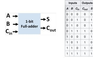
FIG. 8. Schematic drawing for a 1-bit full adder with input carry  $C_{\rm in}$  and output carry  $C_{\rm out}$  and corresponding logical truth table.
