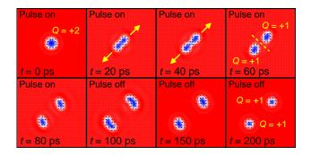
FIG. 4. Out-of-plane current-induced separation of one bilayer skyrmion with  $Q=\pm 2$  to two bilayer skyrmions with  $Q=\pm 1$ . Snapshots are top views of the bottom FM layer. Here, a current pulse of j=400 MA cm<sup>-2</sup> is applied for 100 ps to force the separation.
