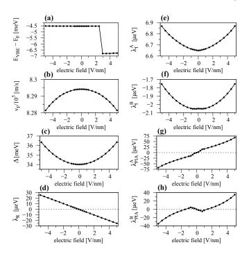
FIG. 20. (Color online) Fit parameters as a function of the applied transverse electric field for the C1 configuration. (a) Valence band edge with respect to the Fermi level, (b) Fermi velocity  $v_{\rm F}$ , (c) gap parameter  $\Delta$ , (d) Rashba SOC parameter  $\lambda_{\rm R}$ , (e,f) intrinsic SOC parameters  $\lambda_{\rm I}^{\rm A}$  and  $\lambda_{\rm I}^{\rm B}$ , and (g,h) PIA SOC parameters  $\lambda_{\rm PIA}^{\rm A}$  and  $\lambda_{\rm PIA}^{\rm B}$ .
