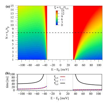
FIG. 22. (Color online) Calculated SR times and anisotropies for C1 configuration and an electric field of 1 V/nm. (a) SR anisotropy  $\xi = \tau_{s,z}/\tau_{s,x}$  as a function of  $N = \tau_{iv}/\tau_p$  and the energy. (b) Individual SR times as a function of energy corresponding to the dashed line in (a) with  $\tau_p = 125$  fs and  $\tau_{iv} = 8 \cdot \tau_p$ . The gray lines indicate the band edges.
