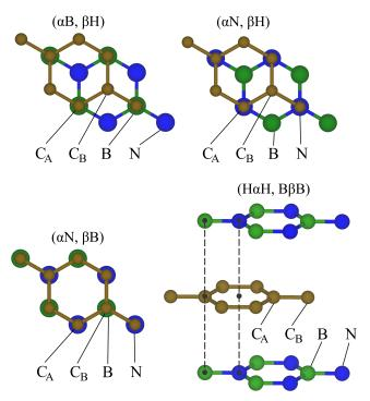
FIG. 1. (Color online) Three high-symmetry commensurate stacking configurations of graphene on hBN,  $(\alpha B, \beta H)$ ,  $(\alpha N, \beta H)$ , and  $(\alpha N, \beta B)$  and the  $(H\alpha H, B\beta B)$  geometry, as an example of hBN encapsulated graphene.
