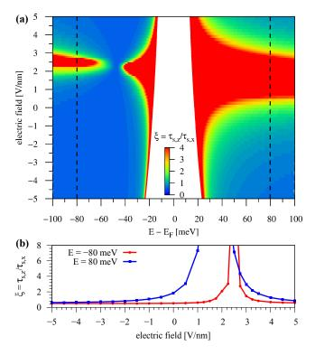
FIG. 13. (Color online) (a) Calculated SR anisotropy  $\xi = \tau_{s,z}/\tau_{s,x}$  as a function of energy and applied transverse electric field for  $(\alpha B, \beta H)$  configuration, using  $\tau_p = 125$  fs and  $\tau_{iv} = 8 \cdot \tau_p$ . (b) Anisotropy  $\xi$  at energies  $E = \pm 80$  meV corresponding to the dashed lines in (a).
