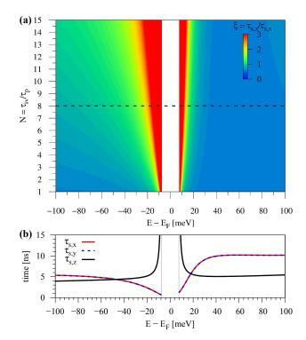
FIG. 12. (Color online) Calculated SR times and anisotropies for graphene on hBN. Here we use the averaged parameters of the graphene/hBN heterostructures given in the main text. (a) Colormap of the SR anisotropy  $\xi = \tau_{s,z}/\tau_{s,x}$  as a function of  $N = \tau_{iv}/\tau_p$  and the energy. (b) Individual SR times as a function of energy corresponding to the dashed line in (a) with  $\tau_p = 125$  fs and  $\tau_{iv} = 8 \cdot \tau_p$ . The gray lines indicate the band edges.
