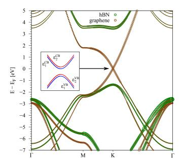
FIG. 2. (Color online) Calculated electronic band structure of the (H $\alpha$ H, B $\beta$ B) geometry, see Fig. 1. The bands of graphene (hBN) are plotted in brown (green). The left inset shows a sketch of the low energy dispersion close to the K point. Due to the presence of the substrate, graphene's low energy bands are split into four states  $\varepsilon_{1/2}^{\mathrm{CB/VB}}$ , with a band gap.
