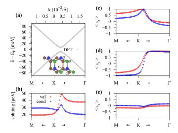
FIG. 15. (Color online) Calculated band properties of graphene on hBN in the vicinity of the K point and an interlayer distance of 3.45 Å. (a) First-principles band structure and local stacking geometry. (b) The splitting of conduction band  $\Delta E_{CB}$  (blue) and valence band  $\Delta E_{VB}$  (red) close to the K point. (c)-(e) The spin expectation values of the bands  $\varepsilon_2^{VB}$  and  $\varepsilon_1^{CB}$ .
