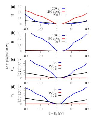
FIG. 14. (Color online) Density of states of graphene on hBN around the Fermi level for  $(\alpha B, \beta H)$  configuration and an interlayer distance of 3.35 Å. The DOS is multiplied by a factor of 100. Each subfigure (a)-(d) correspond to a different atom. For each atom, the orbital contributions to the DOS are multiplied with the corresponding prefactor. The DOS is calculated with a k-point grid of  $180 \times 180 \times 1$ .
