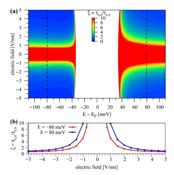
FIG. 23. (Color online) (a) Calculated SR anisotropy  $\xi = \tau_{s,z}/\tau_{s,x}$  as a function of energy and applied transverse electric field for C1 configuration of hBN encapsulated graphene, using  $\tau_p = 125$  fs and  $\tau_{iv} = 8 \cdot \tau_p$ . (b) Anisotropy  $\xi$  at energies  $E = \pm 80$  meV corresponding to the dashed lines in (a).
