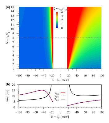
FIG. 11. (Color online) Calculated SR times and anisotropies for  $(\alpha B, \beta H)$  configuration. (a) Colormap of the SR anisotropy  $\xi = \tau_{s,z}/\tau_{s,x}$  as a function of  $N = \tau_{iv}/\tau_p$  and the energy. (b) Individual SR times as a function of energy corresponding to the dashed line in (a) with  $\tau_p = 125$  fs and  $\tau_{iv} = 8 \cdot \tau_p$ . The gray lines indicate the band edges.
