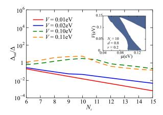
Figure 4: Induced gap as a function of the TI layer thickness  $(N_z)$  for fixed  $\mu = 0.04eV$  and different values of V. Full and dashed lines indicate trivial and topological phases respectively. The relative weight of the inter and intra parity pairing at the bottom layer was fixed to d = 0.8 and r = 0.2. The inset shows the phase diagram in the  $\mu$ -V plane for  $N_z = 10$ .
