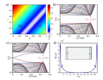
Figure 3: a) Induced gap  $\Delta_{ind}$  in the (d, r) plane for the same parameters as in the lower right panel of Fig. 2. b-c) BdG spectrum for a slab of finite width  $W \sim 20\xi$ , where  $\xi \sim A_2/\Delta$ is the coherence length in the TI film for the cases indicated by the red dots in panel a). As can be observed, subgap states reaching zero energy for  $k_y \to 0$  appear in the topological case. b) Electron probability amplitude for these zero energy states.
