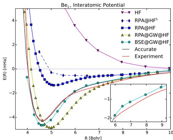
FIG. 2. The interatomic potential of  $\text{Be}_2$ . Red line: experiment [1]; black line: accurate CI [12]; magenta line with triangle down symbols: HF; blue dashed line with diamonds: RPA on top of HF by ACFDT from Ref. [29]; blue line with squares: RPA on top of HF by TF; yellow line with triangle up symbols: RPA on top of GW and HF; cyan line with circles: BSE on top of GW and HF by the TF formula Eq. (6).
