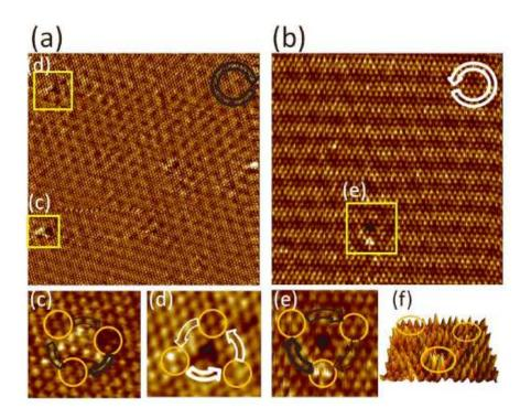
FIG. 5: (a) 24 nm 24 nm STM image measured at 80 K in the clockwise CDW. (b)14 nm 14 nm STM image measured at 8 K in the counterclockwise CDW. The Friedel oscillations in the clockwise CDW [(c) and (e)] and counterclockwise CDW (d). Each peak and gap is indicated by orange circles. The black and the white arrows indicate clockwise and counterclockwise CDWs and FOs, respectively. (f)Three-dimensional plots of (e).
