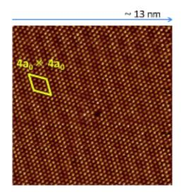
FIG. 1: 13 nm 13 nm STM image measured in situ at a sample voltage of V -100 mV and an initial tunneling current of I 2.0 nA at 80 K. The spots correspond to Se atoms and the brightness corresponds to local electron density. The orange parallelogram indicates the  $4a_0$  4 $a_0$  CDW superlattice.
