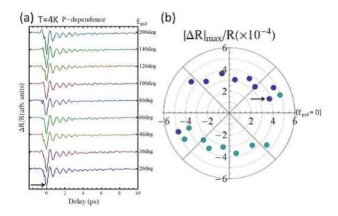
FIG. 4: (a) Polarization dependence of transient reflectivity variation in 1T-VSe<sub>2</sub> measured at 4 K. The hight of each peak is plotted in (b) as a function of polarization angle. The amplitude indicated the black arrows in (a) correspond to the spot indicated that in (b).
