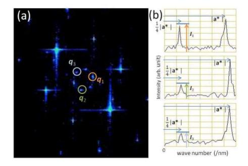
FIG. 2: (a) Fourier transformation (FT) image of Fig. 1. The spots surrounded by circles show the CDW wave vectors  $q_1$ ,  $q_2$  and  $q_3$ . (b) Line profiles along the  $q_1$ ,  $q_2$  and  $q_3$  wave vectors.  $I_1$ ,  $I_2$ and  $I_3$  show the intensities of each CDW peak. FT was performed over the entire field of view (13 nm 13 nm) of the STM image.
