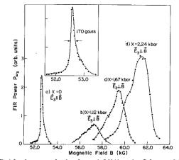
Fig. 3. Far-infrared power as a function of magnetic field (denoted as **B**) for n-type InSb  $(n_e = 5 \times 10^{15} \text{ cm}^{-3})$  at 1.8 K in the X||**B**||[111] geometry. Polarization of the emitted radiation (denoted as **E**<sub>3</sub>) is shown. (a) X = 0, the asymmetric shape of the curve is illustrated in the same inset. (b)–(d) The electric-dipole emission due to k-linear terms of the Hamiltonian for different values of X(Jagannath and Aggarwal 1985).
