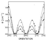
Fig. 8. EDSR intensity as a function of the orientation of H in the (110) plane for  $q \parallel [110]$ (longitudinal Voigt geometry). Black and white circles correspond to opposite signs of H. respectively. The solid line is the theoretical angular dependence of EDSR (Rashba and Sheka 1961a). The dashed curves are guides for the eve, connecting experimental points (Dobrowolska et al. 1983).
