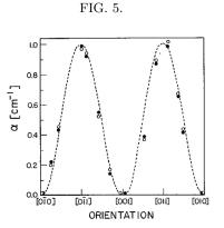
Fig. 6. EDSR intensity in n-type InSb as a function of the orientation of H in the (100) plane. Black and white dots indicate opposite orientations of the field. The dashed line is the theoretical depe dence for this plane (Rashba and Sheka 1961a), normalized to the experimental data for H [011]. The data were observed at 4.5 K at 118.8  $\mu$ m on a sample with  $n_c = 3.6 \times 10^{14} \text{ cm}^{-3}$ , 4 mm thick (Dobrowolska et al. 1983).
