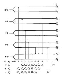
Fig. 5. Scheme of COR transitions in n-type InSb for the inversion asymmetry mechanism (g < 0) Under the transition the respective values of  $\Delta m$  and of the intensity indicatrix for all polarizations  $\tau$ are given. The transitions with  $\Delta N = 3$  and  $\Delta N = 4$  are forbidden in the Zeeman limit for the Hamiltonian (6.2). Polarizations in which CR and EPR are excited are also indicated, their indicatrices being isotropic.
