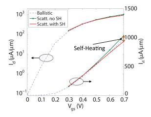
FIG. 4. (Color online) Transfer characteristics  $I_d$ - $V_{gs}$  at  $V_{ds}=0.67$  V of the single-gate transistor in Fig. 1 with a single-layer MoS<sub>2</sub> as channel. The ballistic limit of transport (dashed blue lines), the current with electron-phonon scattering, but an equilibrium phonon population (green lines with crosses), and the current with self-heating effects (solid red lines) are provided. The current reduction caused by self-heating is indicated by the orange double-arrow.
