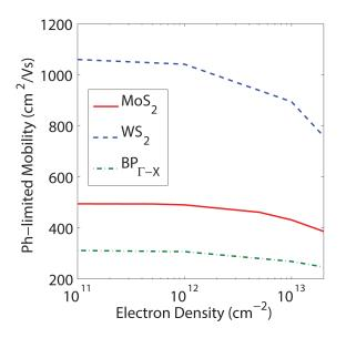
FIG. 9. (Color online) Electron phonon-limited mobility of single-layer  $MoS_2$ ,  $WS_2$ , and AC BP as a function of the carrier concentration<sup>49</sup> and with the same plotting conventions as in Fig. 3. The "dR/dL" mobility extraction method has been used for that purpose<sup>48</sup>.
