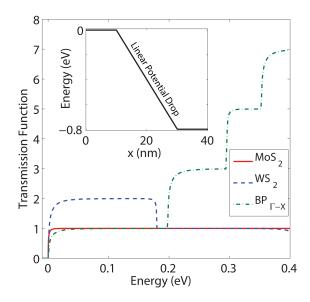
FIG. 5. (Color online) Electron transmission function, as obtained from quantum transport calculations, through the same single-layer 2-D materials as in Fig. 3 at  $k_z=0$ , but with a linear potential drop (see inset) between both structure ends instead of flat band conditions.
