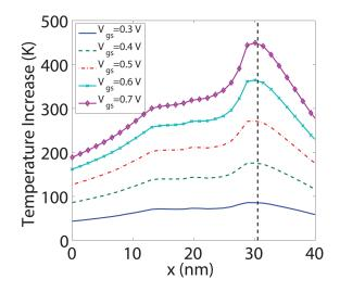
FIG. 7. (Color online) Effective lattice temperature increase  $\Delta T = T - T_0$  as a function of the position along the x-axis and of the gate voltage  $V_{gs}$  at a fixed drain bias  $V_{ds} = 0.67$  V for the same single-layer MoS<sub>2</sub> transistor as in Fig. 6.
