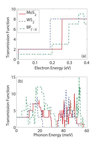
FIG. 3. (Color online) (a) Electron transmission function, as obtained from quantum transport calculations, through single-layer MoS<sub>2</sub> (solid red line), WS<sub>2</sub> (dashed blue line), and AC BP (dasheddotted green line) at  $k_z=0$ , with flat-band conditions, and with the conduction band minimum aligned with the energy E=0 eV. (b) Same as (a), but for phonons at  $q_z=0$ .
