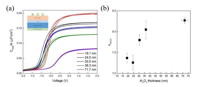
FIG. 2. (a) C–V curves achieved for the different capacitors, with different thicknesses of Al<sub>2</sub>O<sub>3</sub> layer, normalized to the measured contact area measured at 1 MHz; inset: Schematic description of the MOS capacitors used to determine the dielectric constants of Al<sub>2</sub>O<sub>3</sub> films (b) Dependence of the dielectric constant on thickness of the Al<sub>2</sub>O<sub>3</sub> layer
