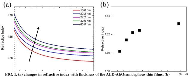
dependence of refractive index on thickness of the amorphous Al<sub>2</sub>O<sub>3</sub> layer
