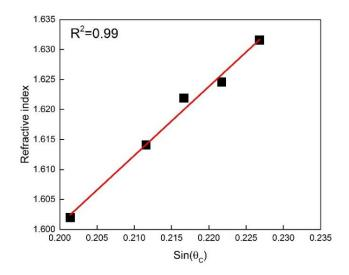
FIG. 3. Relationship between the critical angle (measured by XRR) and the refractive index (measured by ellipsometry)
