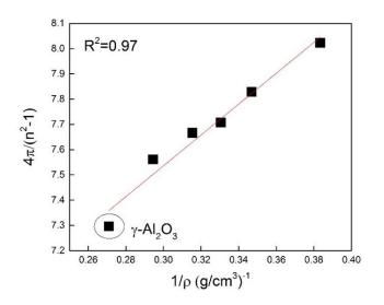
FIG. 4. Dependence of the refractive index on density, according to Anderson and Schreiber
