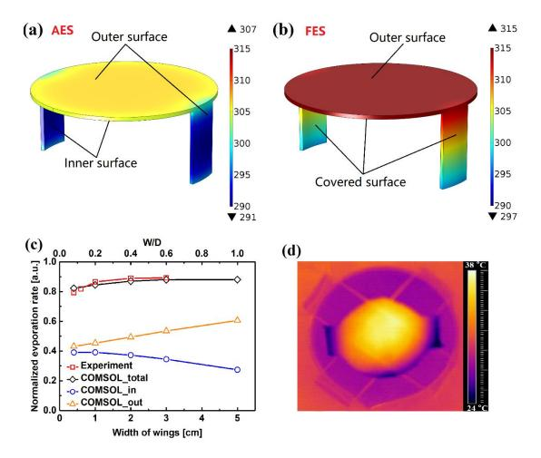
Figure 4 (a) The water temperature in AES for width of wings at 1 cm. The outer (inner) surface indicates that the vapor diffusion near the surface isn't (is) blocked by the wings.(b) The temperature distribution of water in FES for the width of wings at 1 cm. The covered surface means the surface is covered by insulating material. (c) The normalized evaporation rate of AES. "Total" indicates the total evaporation rate, "in" and "out"
