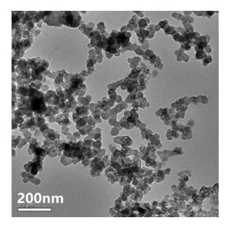
Figure 2. The TEM image of the carbon black nanoparticles. The scale bar is 200 nm.
