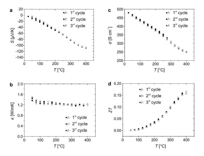
**Fig. 5.** Thermoelectric characterization of  $Mn_{o.85}Bi_{2.1}Te_4$  ingot measured in three consecutive cycles. a) Seebeck coefficient S. b) thermal conductivity κ. c) electrical conductivity σ. d) thermoelectric figure of merit ZT as a function of temperature. Filled symbols: heating, open symbols: cooling.
