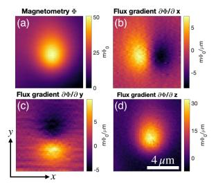
FIG. 3. (a) Magnetometry image of a vortex in a Nb film, measured with a 0.6  $\mu$ m inner diameter pickup loop.<sup>22</sup> (b,c) Numerical gradients of the flux data from (a) in the *x* and *y* directions, respectively. (d) *z*-gradient of the flux, calculated from magnetometry maps at two heights above the Nb film, separated by  $\Delta z = 0.4 \,\mu$ m.
