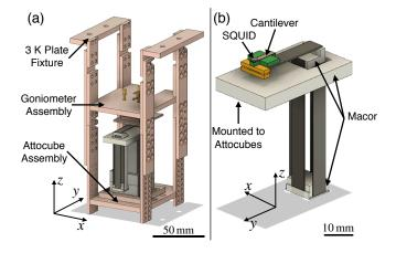
FIG. 1. (a) CAD model of fully assembled cage. (b) CAD model of the piezoelectric scanner, with the SQUID sensor at the end of the *z*-axis piezo bender. The large Macor section of the scanner is mounted rigidly to the Attocube stack for coarse positioning.
