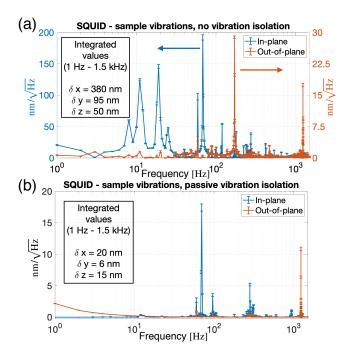
FIG. 5. Sensor-sample vibration spectrum up to 1.5 kHz before (a) and after (b) implementation of passive vibration isolation, extracted from fits to SQUID noise near an isolated vortex (see Appendix A). Insets: Sensor-sample displacement along the x, y, and z axes, integrated from 1 Hz to 1.5 kHz. Error bars are 95% confidence intervals from least squares fitting.
