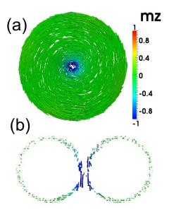
Figure 5: Fig. a shows the magnetization field obtained from micromagnetic simulations for a nanotorus with R = 100 nm and r = 99 nm, seen from top. Fig. b) presents a cross section in the center of the nanotorus aiming to show the components of the magnetization pointing along the out-of-plane direction.
