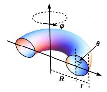
Figure 1: Toroidal geometry and parameters describing a torus shell. R and r are the external and internal radii respectively and  $\varphi$  and  $\theta$  ( $\in$   $[0,2\pi)$ ) are the azimuthal and polar angles, respectively.
