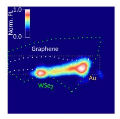
Supplementary Figure 2 | Photoluminescence map at 300 K (WSe<sub>2</sub> sample). Photoluminescence from monolayer WSe<sub>2</sub> at room temperature (excitation  $\lambda = 532$  nm,  $P_d = 8 \times 10^3$  W cm<sup>-2</sup>). The PL is quenched on graphene.
