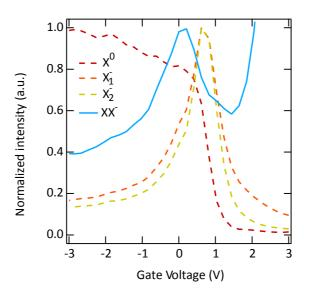
Supplementary Figure 5 | PL emission from exciton complexes as a function of external electric field in WS<sub>2</sub>. Line-cut of the normalized PL intensity of different exciton species as a function of doping level. In the highly n-doped regime ( $V_G > 2 V$ ), where X<sup>0</sup> (red), X<sub>1</sub><sup>-</sup> (orange), X<sub>2</sub><sup>-</sup> (yellow), XX<sup>-</sup> (blue) species vanish, the next charging state of the trion may be observed, as in WSe<sub>2</sub><sup>3</sup>.
