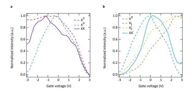
Supplementary Figure 4 | PL emission from exciton complexes as a function of external electric field in WSe<sub>2</sub>. Line-cut of the normalized PL intensity of different exciton species. **a**, Biexcitons (purple) **b**, charged biexcitons (blue) as a function of doping level. The behavior of the different peaks with the back voltage is in good agreement with recently reported results<sup>1–4</sup>.
