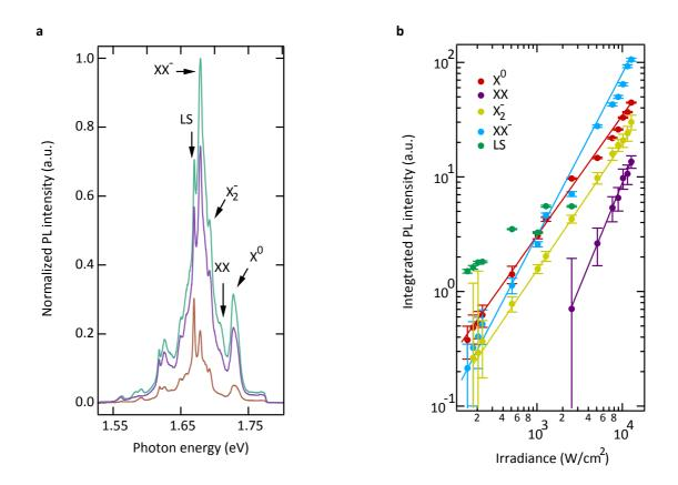
Supplementary Figure 6 | Power-dependence of the PL intensity in WSe<sub>2</sub>. a, PL spectra of a WSe<sub>2</sub> monolayer for different excitation intensities ( $P_d$  = 2.5x10<sup>3</sup> Wcm<sup>-2</sup> to 1.2x10<sup>4</sup> Wcm<sup>-2</sup>). b, Logarithmic plot of the integrated PL intensity as a function of the excitation intensity. Circles represent the experimental data, while lines
