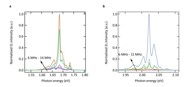
**Supplementary Figure 9 | EL intensity as a function of the pulse frequency. a,** WSe<sub>2</sub> EL spectra at frequencies ranging from 6 MHz to 14 MHz. **b,** WS<sub>2</sub> EL spectra at frequencies ranging from 6 MHz to 11 MHz. The emission intensity increases with frequency, in agreement with similar measurements performed at room temperature<sup>13</sup>. Furthermore, all the emission peaks broaden at higher frequencies.
