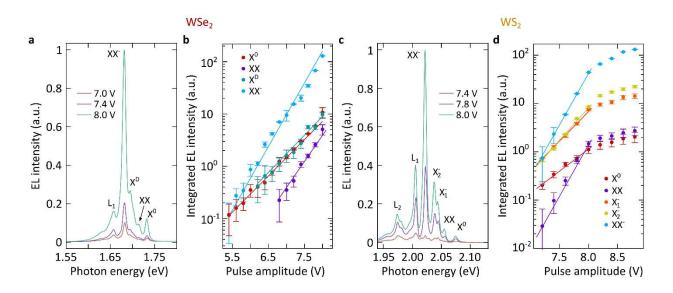
**Figure 3** | **EL intensity dependence with the excitation power. a**, Pulsed EL emission spectra of WSe<sub>2</sub> for different pulse amplitudes and fixed offset voltage. b, Semi-logarithmic plot of the integrated EL intensity as a function of the pulse amplitude. The circles represent the experimental data, while the lines depict the fit to an exponential function as discussed in the main text. c, and **d**, Same as in a, and b, but for WS<sub>2</sub>.
