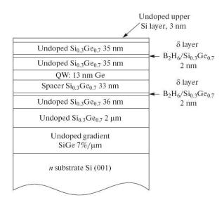
FIG. 3. Structure of sample no. 1.
