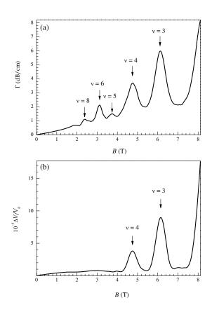
FIG. 4. Dependences  $\Gamma(B)$  (a),  $\Delta V/V(B)$  (b), f=142 MHz, T=4.2 K,  $\nu$  is the filling factor
