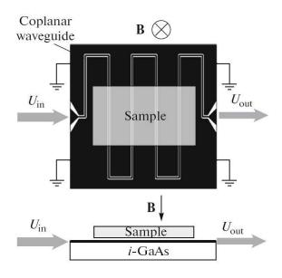
FIG. 2. Sketch of the microwave technique.
