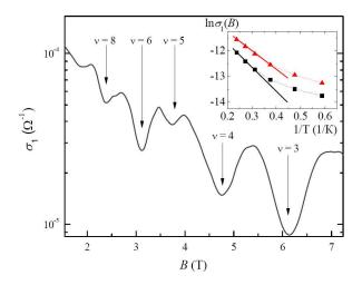
FIG. 5. Dependence  $\sigma_1(B)$  for frequency f=142 MHz at T=4.2 K;  $\nu$  is the filling factor. The inset shows the dependence of  $\ln \sigma_1(B)$  on inverse temperature at oscillation minima with filling factor  $\nu=3$  (squares) and 4 (triangles).
