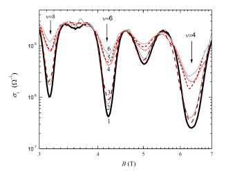
FIG. 10. Dependences of  $\sigma_1$  on at different frequencies f, MHz: (1) 30, (3) 197 (acoustic method); (2) 148, (4) 585, (5) 906, and (6) 1191 (microwave technique); T=1.7 K; sample no. 2.
