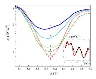
FIG. 8. Dependences  $\sigma_1(B)$  for different frequencies: (1) 30MHz and (2) 142 MHz (acoustic method); (3) 250 MHz, (4) 328 MHz, (5) 800 MHz, and (6) 1130 MHz (microwave technique); T = 4.2 K. The inset shows the  $\sigma_1(B)$  dependences obtained by superposition of curves for  $f \approx 220$  MHz; solid and dashed curves correspond to the microwave and acoustic techniques.
