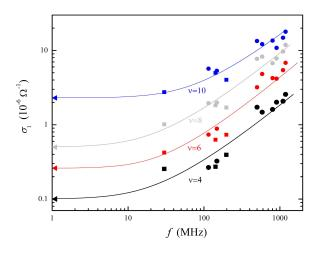
FIG. 11. Dependences  $\sigma_1(f)$  at the minima of oscillations with  $\nu = 4, 6, 8, 10$ . Squares correspond to acoustic method, circles are the data obtained by microwave technique, and triangles correspond to  $\sigma_{\rm D}, T=1.7$  K.
