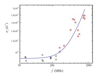
FIG. 9. Dependences  $\sigma_1(f)$  at the minimum with filling factor  $\nu=3$  at T=4.2 K;  $\bigcirc$  are the data obtained using the acoustic method;  $\Box$  correspond to the microwave technique. The solid scaling curve — is drawn in accordance with the theory described in Section 4.
