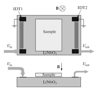
FIG. 1. Illustration the acoustic method. A SAW is generated by interdigital transducer 1 (IDT1) and is detected by IDT2 after the passage over the surface of the LiNbO3 piezoelectric substrate.
