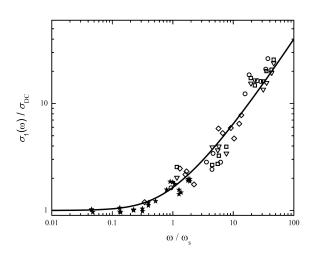
FIG. 12. Dependence of  $\sigma_1/\sigma_{DC}$  on  $\omega/\omega_S$ :  $\bigstar$  correspond to sample no. 1 (T=4.2 K),  $\Box$  correspond to sample no. 2,  $\nu=4$ ;  $\bigcirc$ , sample no. 2,  $\nu=6$ ;  $\bigtriangledown$ , sample no. 2,  $\nu=8$ ;  $\diamondsuit$ , sample no. 2,  $\nu=10$ .
