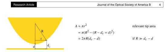
Fig. 2. Sketch of the tip area that contributes to the anomalous heat transfer.
