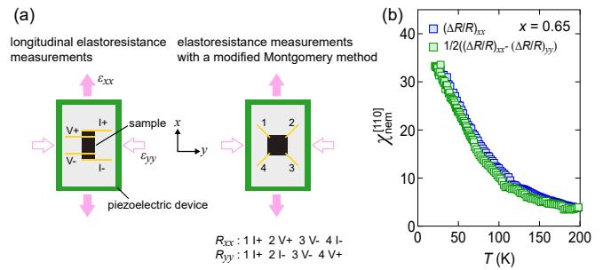
FIG. 6. Biaxial strain effect to the nematic susceptibility. (a) Schematic illustration of the two elastoresistance measurements. (b), The temperature dependence of  $\chi_{\text{nem}}^{[110]}$  for  $\text{Ba}_{1-x}\text{Rb}_x\text{Fe}_2\text{As}_2$  with  $x = 0.65$  obtained by longitudinal elastoresistance measurements (blue square), which is the same data as in Fig. 3(a), and by a modified Montgomery method (green square).
