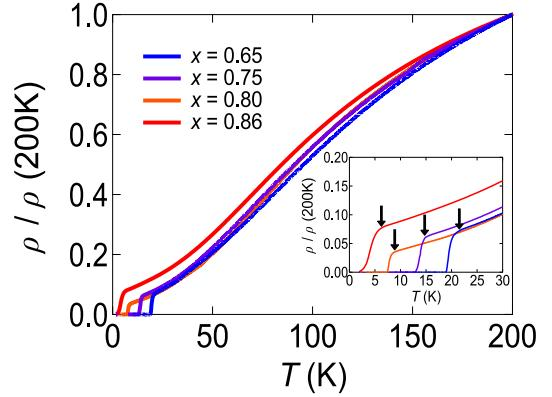
FIG. 5. Temperature dependence of the resistivity for the  $\text{Ba}_{1-x}\text{Rb}_x\text{Fe}_2\text{As}_2$  single crystals. The vertical axis is normalized by the resistivity value at 200 K. The inset shows an expanded view below 30 K. The arrows indicate the onset of superconducting transition.
