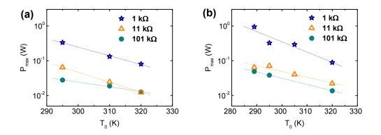
**Figure 3.** The peak power  $P_{max}$  at switching versus ambient temperature  $T_0$  for crystals D5(3) (a) and D3(11) (b) connected to the different load resistances  $R_L$ .
