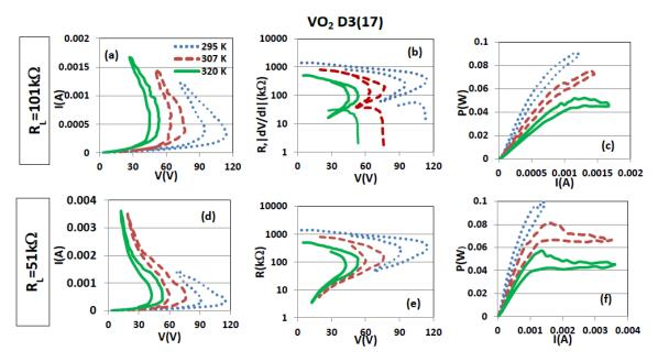
**Figure S5.** I(V), R(V)(=V/I) and P(V)(=VI) for sample D3(17) at temperatures 295, 307 and 320 K (see legend on frame (a)) with  $R_L=101 \text{ k}\Omega$  ((a) –(c)) and  $R_L=51\text{k}\Omega$  ((d) –(f)). |dV/dI|(V) in the NDR regime is shown in (b) below R(V).
