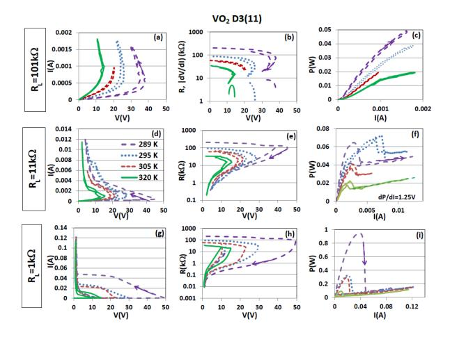
**Figure S3.** I(V), R(V)(=V/I) and P(V)(=VI) for sample D3(11) at temperatures 289, 295, 305 and 320 K (see legend on frame (d)) with  $R_L=101 \text{ k}\Omega$  ((a) –(c)),  $R_L=11\text{k}\Omega$  ((d) –(f)) and  $R_L=1\text{k}\Omega$  ((g)-(i)). |dV/dI|(V) in the NDR regime is shown in (b) below R(V).
