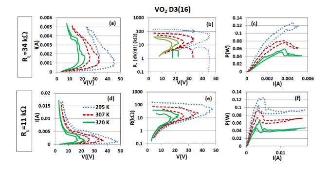
**Figure S4.** I(V), R(V)(=V/I) and P(V)(=VI) for sample D3(16) at temperatures 295, 307 and 320 K (see legend on frame (d)) with  $R_L=34 \text{ k}\Omega$  ((a) –(c)) and  $R_L=11\text{k}\Omega$  ((d) –(f)). |dV/dI|(V) in the NDR regime is shown in (b) below R(V).
