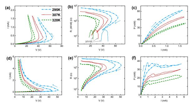
**Figure 4.** I(V), R(V)(=V/I) and P(V)(=VI) for sample D5(4) at temperatures 295 K, 307 K and 320 K [see legend in panel (a)] with  $R_L=101 \text{ k}\Omega$  [(a) –(c)] and  $R_L=34\text{k}\Omega$  [(d) –(f)]. |dV/dI|(V) in the NDR regime is shown in (b) below R(V). Arrows indicate the scan direction.
