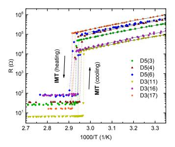
**Figure 1.** Two-contact resistance: R versus 1000/T for crystals D5(3), D5(4), D5(6), D3(11), D3(16) and D3(17).
