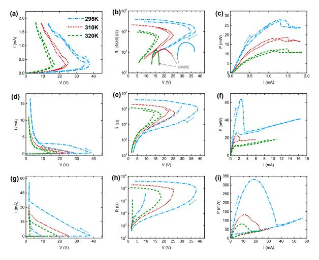
**Figure 2.** I(V), R(V)(=V/I) and P(V)(=VI) for sample D5(3) at temperatures 295, 310 and 320 K [see legend on frame (a)] with R<sub>L</sub>=101 k $\Omega$  [(a) –(c)], R<sub>L</sub>=11k $\Omega$  [(d) –(f)] and R<sub>L</sub>=1 k $\Omega$  [(g)-(i)]. |dV/dI|(V) in the NDR regime is shown in (b) below R(V). Arrows indicate the scan direction.
