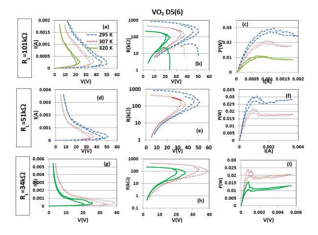
**Figure S6.** I(V), R(V)(=V/I) and P(V)(=VI) for sample D5(6) at temperatures 295, 307 and 320 K (see legend on frame (a) with  $R_L < |dV/dI|_{max}$  at all temperatures.
