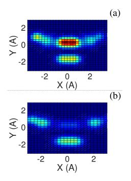
FIG. 2. Electroluminiscence profile in a MBDT molecular junction (Fig. 1b) at  $V_{sd} = 3$  V. The profile is plotted parallel to the molecule at 1.5 Å above the molecular plane. The horizontal axis (X) is the direction of tunneling in the junction. The localized surface plasmon-polariton vector is assumed to be directed along X. The light emission profiles are shown for the outgoing photons of frequencies (a)  $\omega = 2$  eV and (b) 3 eV.
