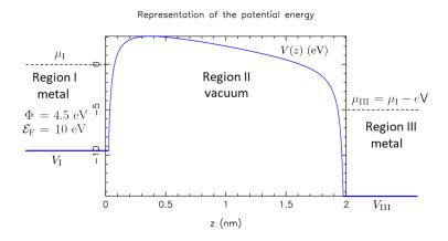
FIG. 1. Potential energy in a metal-vacuum-metal junction. A static voltage V of 5 V is applied. The gap spacing D is 2 nm. We take for convenience the Fermi level  $\mu_{\rm I}$  of the left-side metal as reference for the potential-energy values.
