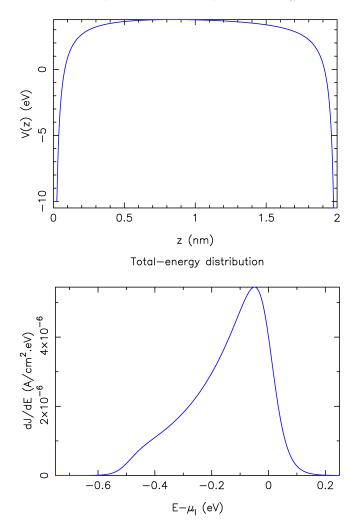
FIG. 2. Potential energy V(z) (top) and total-energy distribution of the current density dJ/dE (bottom) for an applied voltage V of 0.5 V. dJ/dE is calculated by the transfer-matrix technique. We take for convenience the Fermi level  $\mu_{\rm I}$  of the left-side metal as reference for the potential-energy values.
