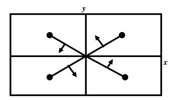
FIG. 1: The nearest neighbors in the Mn and Fe monolayers on the W(110) plane. The lines and arrows are the n.n. bonds and DM vectors. The lattice constants along x and y axes are  $\sqrt{2}$  and unity respectively.
