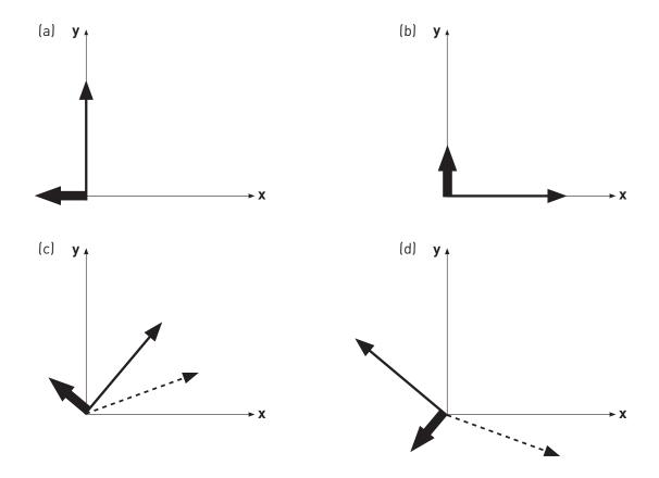
FIG. 2: The field dependence of the  $(\hat{c}, \mathbf{k})$  orientation. (a)  $\Psi = 0$ ,  $H < H_{ac}$ . (b)  $\Psi = 0$ ,  $H > H_{ac}$ . (c)  $\Psi > 0$ . (d)  $\Psi < 0$ . Thin, thick and dashed arrows are  $\hat{c}$ ,  $\mathbf{k}$  and  $\mathbf{H}$  respectively.
