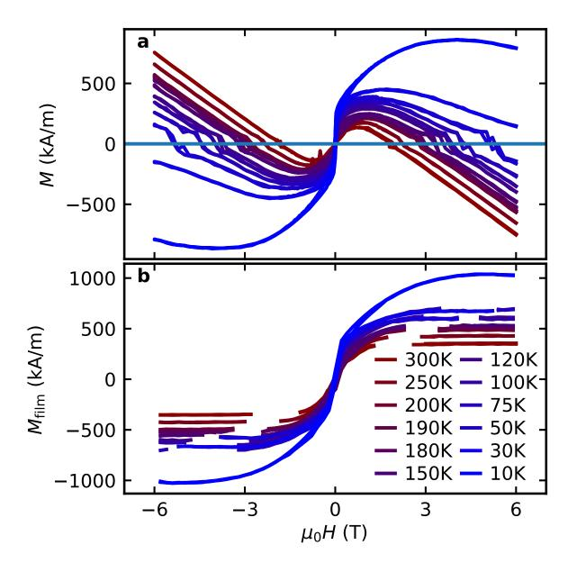
Figure 2: **a** The out-of-plane magnetization measurements of the  $Mn_{1.8}PtSn$  thin film goes through zero at finite fields due to the diamagnetic substrate contribution, giving rise to measurement artifacts. Therefore, the zero crossings have been masked. **b** Out-of-plane magnetization with subtracted background as used for the extraction of the topological Hall and Nernst effect.
