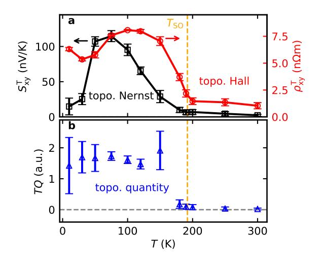
Figure 3: **a** The maximum amplitudes of the topological Nernst and Hall signals are shown by black and red symbols, respectively. In contrast to the THE, the TNE decreases by at least a factor of 8 towards low temperatures (T < 50 K). **b** The maximum of the topological quantity (TQ) decreases to 0 within the experimental error above  $T_{\text{SR}}$  (marked by the orange line). Interestingly, the topological Hall and Nernst effect do not seem to completely vanish above  $T_{\text{SR}}$ .
