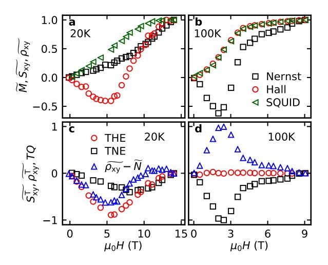
Figure 5: **a,b** Normalized Nernst  $\widetilde{S}_{xy} = S_{xy}/\max(S_{xy})$ , Hall  $\widetilde{\rho}_{xy} = \rho_{xy}/\max(\rho_{xy})$  and SQUID magnetometry  $\widetilde{M} = M/\max(M)$  measurements for bulk MnGe as reported in Ref.<sup>7</sup> **c,d** The extracted topological quantity TQ (blue triangles) also for this sample reflects the region where either topological Hall or Nernst are observed.
