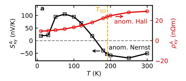
Figure 4: **a** The saturation values of the Nernst (black squares) and Hall (red circles) signals, i.e. the anomalous Hall and Nernst signals both show a dependence on temperature: While the AHE only decreases towards lower temperatures, the ANE changes its sign below the spin reorientation temperature.
