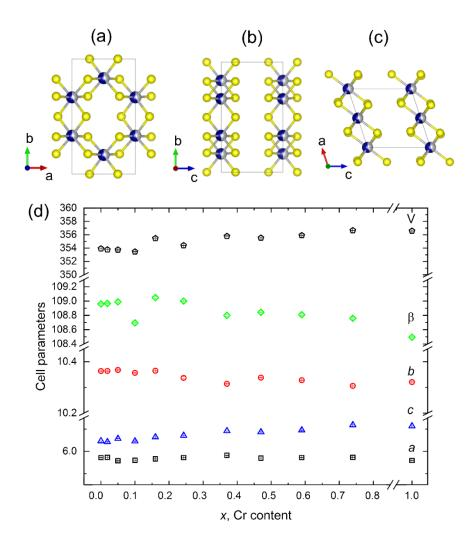
**Figure 3.** Crystal structure and lattice parameters for the  $Ru_{1-x}Cr_xCl_3$  series. Ru, Cr and Cl atoms are shown in blue, gray and yellow, respectively.
