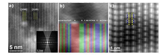
**Figure 7.** (a) HR-STEM image of the Ru<sub>0.91(4)</sub>Cr<sub>0.10(2)</sub>Cl<sub>3</sub> sample taken along the 100 zone-axis with overlaid atomic structure for the 100 and 110 zone axis. Inset shows the FFT of the image and the marked mask for filtered image b. (b) Fourier filtered image of a, with color coded and marked stacking sequences. (c) Close-up of the atomic structure with of an atomic overlay of the 100 zone axis, blue and yellow circles denote Ru/Cr and Cl columns, respectively.
