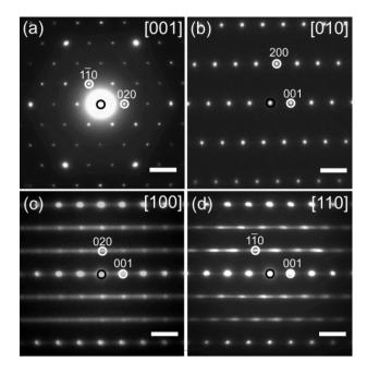
**Figure 5.** Electron diffraction patterns of a  $Ru_{0.91(4)}Cr_{0.10(2)}Cl_3$  sample along the (a) 001, (b) 010, (c) 100, and (d) 110 zone-axis directions. The scale bar corresponds to 2 nm<sup>-1</sup>.
