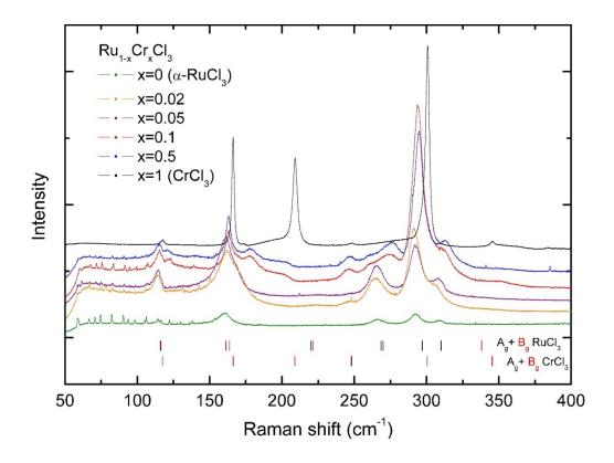
**Figure 8.** Raman spectra of the  $Ru_{1-x}Cr_xCl_3$  series recorded with an excitation wavelength of 633 nm.
