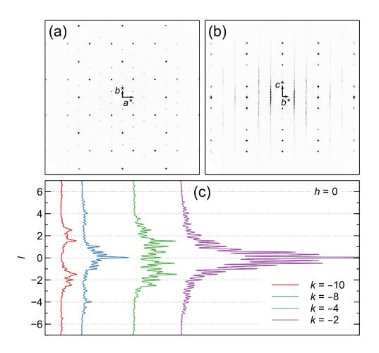
**Figure 4.** Re-calculated reciprocal layers (a) hk0 and (b) 0kl of Ru<sub>0.91(4)</sub>Cr<sub>0.10(2)</sub>Cl<sub>3</sub>; the intensity distribution along the series containing diffuse contributions exhibit a certain modulation pointing towards partial ordering (c).
