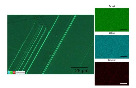
**Figure 2.** Secondary electron (SE) image and EDX color maps from a representative Ru/Cr mixed metal  $Ru_{0.91(4)}Cr_{0.10(2)}Cl_3$ . The scale bar corresponds to 25 µm.
