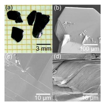
**Figure 1.** (a)  $\operatorname{Ru}_{1-x}\operatorname{Cr}_x\operatorname{Cl}_3$  crystals grown by chemical vapor transport (b–d) Scanning electron micrographs taken at 2.0 keV in the SE mode showing the morphology of the  $\operatorname{Ru}_{1-x}\operatorname{Cr}_x\operatorname{Cl}_3$  crystals in the *ab*-plane and along the stacking fault direction.
