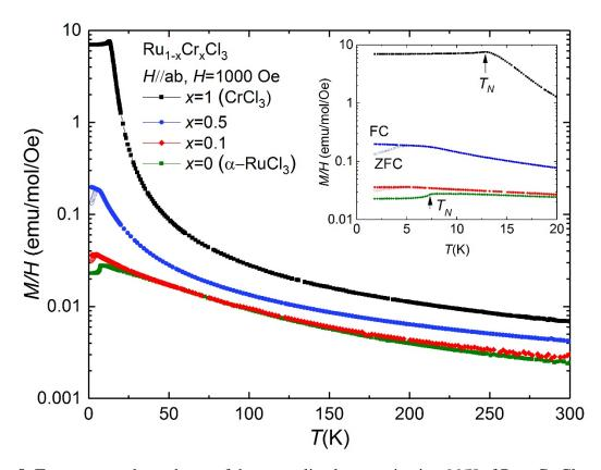
**Figure 9.** Temperature dependence of the normalized magnetization M/H of Ru<sub>1-x</sub>Cr<sub>x</sub>Cl<sub>3</sub> on a semi-logarithmic scale. The magnetic field of 1000 Oe was applied in the *ab* plane of Ru<sub>1-x</sub>Cr<sub>x</sub>Cl<sub>3</sub> single crystals. The inset is a zoom into the low-temperature region. Open and full symbols stand for zero-field-cooled (ZFC) and field-cooled (FC) magnetization measurements.
