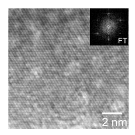
**Figure 6.** TEM image of Ru<sub>0.91(4)</sub>Cr<sub>0.10(2)</sub>Cl<sub>3</sub> sample taken in the 001 zone-axis and the corresponding FFT.
