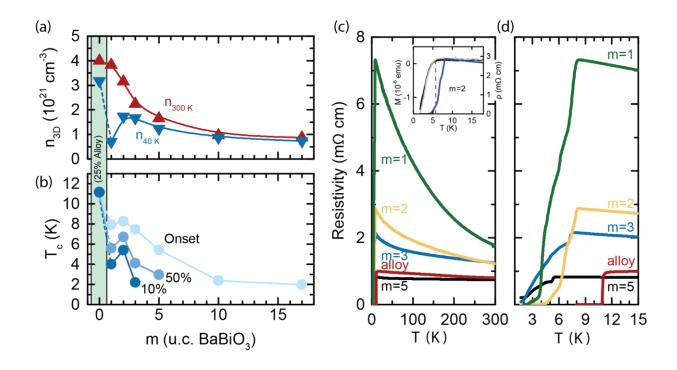
**Figure 3.** Transport characterization. (a) Room and low temperature 3D carrier densities extracted from Hall measurements. (b) Transition temperatures extracted from resistivity measurements. (c) Full temperature range resistivity vs. temperature. The inset of (c) overlays the transition probed by resistive measurements (blue) with out-of-plane (black) and in-plane (grey) onset of diamagnetism (red dashed line) for m=2. (d) Transition region of superconducting samples.
