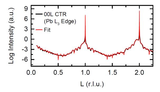
**Figure 5.** Experimentally measured and the COBRA simulated specular (00L) crystal truncation rod with the X-ray energy tuned to just below the Pb L<sub>3</sub> absorption edge.
