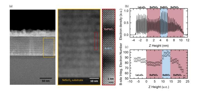
**Figure 2.** TEM characterization of BaBiO<sub>3</sub>/BaPbO<sub>3</sub> and chemical interfacial width and intermixing at the interfaces resolved by the resonant coherent Bragg rod analysis method. (a) Low and high resolution STEM images. (b) Resonant COBRA-derived electron density profile of a BaPbO<sub>3</sub>/BaBiO<sub>3</sub>/BaPbO<sub>3</sub> trilayer sample. (c) Resonant COBRA-derived integrated electron number in each perovskite B-site atomic layer along the out-of-plane direction.
