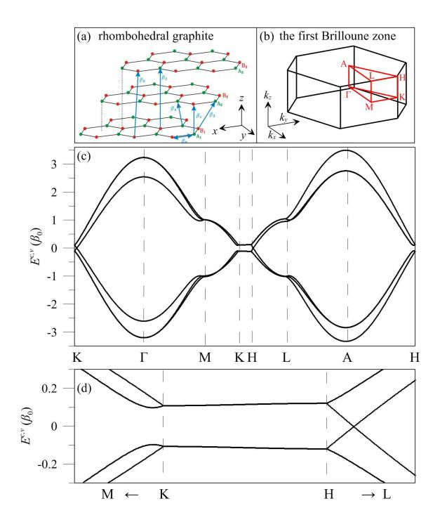
Figure 1: The geometric structure (a), the first Brilloune zone (b), and the wholeenergy/low-lying band structures (c)/(d) of the rhombohedral graphite.
