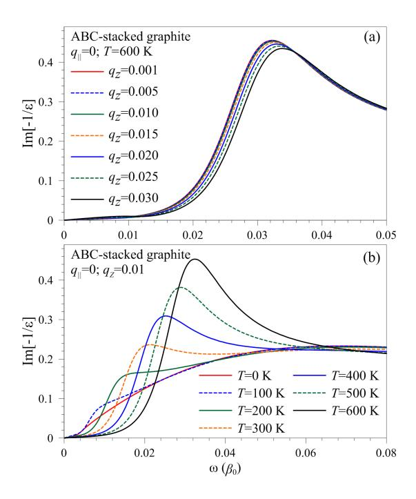
Figure 4: The energy loss function for the ABC-stacked graphite under the conditions: T=600 K & various  $q_z$ s, and  $q_z=0.01$  Å<sup>-1</sup> and different temperatures, being shown in (a) and (b), respectively.
