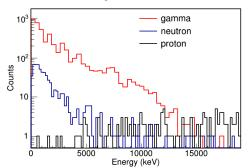
Fig. 7 Energy spectra of particles entering the image sensor recorded during proton simulation runs.
