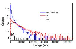
Fig. 6 Energy spectra of particles entering the image sensor recorded during electron simulation runs.
