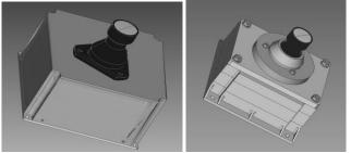
Fig. 4 JUICE camera before (left) and after (right) shielding optimization.
