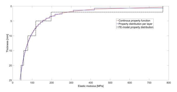
Figure 8: Variation of elastic modulus, E, through a FG model-ice sheet (von Bock und Polach, 2015), determined by the means of experiments (von Bock und Polach et al. 2013) and a numerical model (von Bock und Polach 2015)
