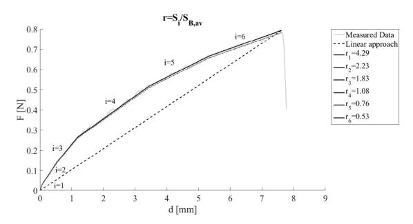
Figure 5: Piece-wise linearization of the load deflection curve under bending for columnar model ice. The legend also contains the stiffness ratio between the individual piecewise linear section and the "linear approach" (Gralher 2017)
