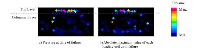
Figure 7: Pressure distribution in columnar-grained model ice under uniaxial compression with columnar model ice doped with sodium-chloride (Gralher 2017).
