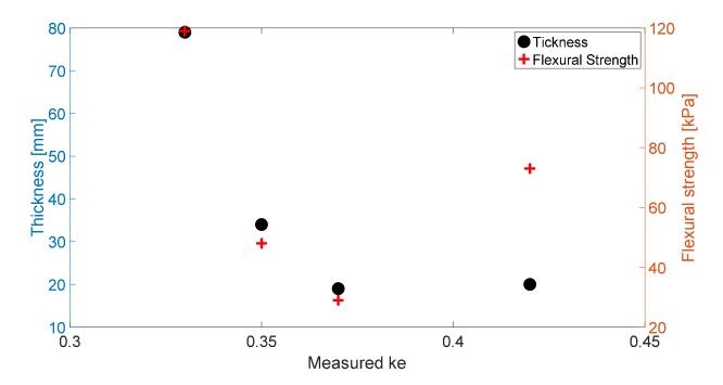
Figure 14: Dependency of the measured bulk partition coefficient (ke) on the ice thickness and the flexural strength for columnar model ice grown from saline doped water (here data from HSVA).
