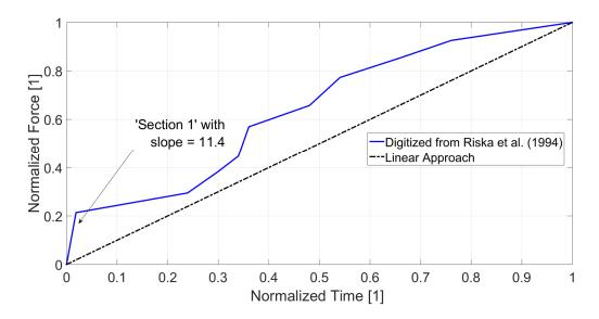
Figure 6: Normalized force-time plot of a digitized cantilever beam test (Figure 17) from Riska et al. (1994) and the Linear Approach proposed by Gralher (2017).
