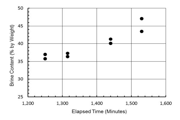
Figure 15: The time variation of urea brine content in ice beams obtained from the ice sheet during the warming period, which began at zero minutes. The two measurement points refer to two examined ice beams cut from the ice sheet (Cook 1983).
