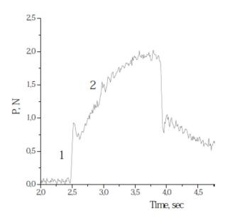
Figure 4: Force-time progression of a cantilever beam test with granular ice at the Krylov State research Centre, adapted from Sazonov and Kelementeva (2011).
