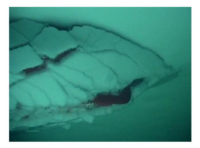
*Figure 1: Underwater view of ice-breaking pattern with model-ice failing in downward flexure (courtesy of HSVA)*
