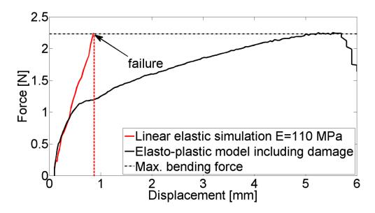
Figure 3: Comparison of the simulation with the elasto-plastic model which represents the experiments and a linear elastic cantilever beam with properties derived from plate deflection tests (von Bock und Polach 2016).
