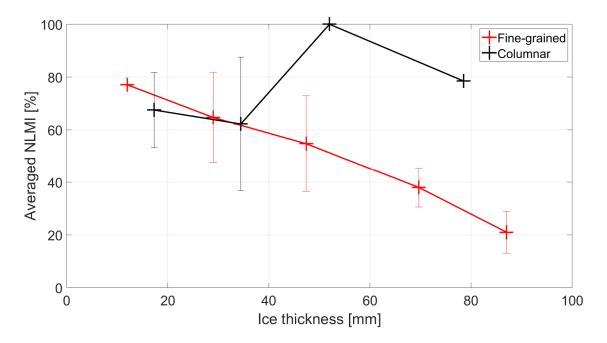
Figure 11: Average NLMI values for fine grained and columnar ice. Each marked point reflects the averaged thickness and NLMI values over the ranges marked by the grind lines of the horizontal axis. The error bars reflect the standard deviation i.e. the scatter at the particular points.
