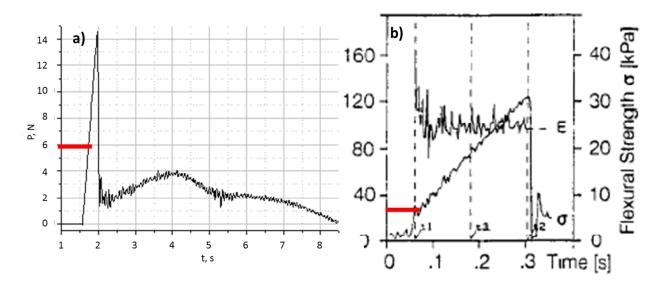
Figure 12: a) Force-time curve of a cantilever beam test of a granular NaCl doped ice, in 87 mm thick ice with a flexural strength,  $\sigma_f = 28,2 \text{ kPa}$  and a low non-linearity, NLMI, of 15%, (measured at KSRC, 2018). b) Force-time curve of a cantilever beam test of columnar NaCl doped ice, in 31 mm thick ice with a flexural strength,  $\sigma_f = 31 \text{ kPa}$  and a high non-linearity, NLMI, of 95% (from Evers and Jochmann 1993).
