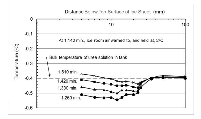
*Figure 16: The warming of the same ice sheet as in Figure 15 was with 2°C room temperature from 1,140-1,520 minutes for the 30 mm thick ice sheet (Cook, 1983).*
