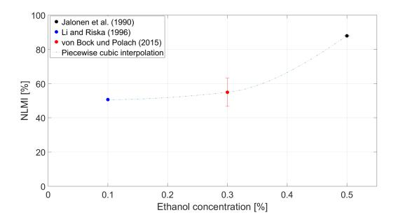
Figure 13: NLMI in dependence on the concentration of the dopant ethanol in tank water.
