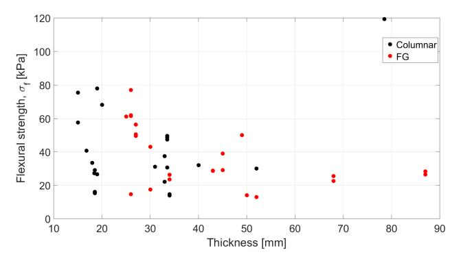
*Figure 9: Columnar and fine grained (FG) force-time data of flexural strength measurements for which thickness and flexural strength are available.*
