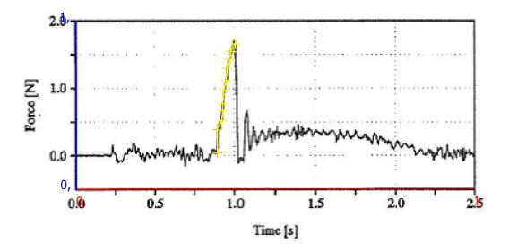
Figure 17: Force-time plot of a cantilever beam test with FG-X ice taken from Riska et al. (1994) after plot digitalization (with yellow markers). The ice thickness is 30 mm and the flexural strength 43 kPa.
