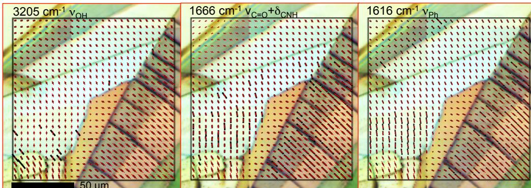
Figure 8: Overlaid optical cross-polarised images of paracetamol form II and vector maps of orientation of the absorption  $\theta'$  (black-bars) at several absorbance bands with the optical slow-axis (retardance azimuth)  $\theta'_n$  (red-bars) measured at  $3600\text{ cm}^{-1}$  where is no absorption. The band  $\nu_{Ph}$  is C=O, C=C stretching of the aromatic ring [19]. See details of statistical analysis for the  $3205\text{ cm}^{-1}$  band in Sec. Appendix A Fig. A.1.
