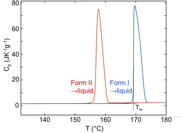
Figure 3: Specific heat capacity  $c_p$  measured on heating at the rate of 10 K/min for the specimen as purchased (in the first heating, blue line) and after cooling at 10 K/min (in the second heating, red line). The highest temperature reached at the end of the first cycle was 180°C.
