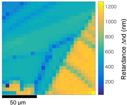
Figure 6: Retardance  $\Delta nd$  map of the same area shown in IR absorbance analysis in Fig. 5 at  $3600\text{ cm}^{-1}$ . The pixel pitch was  $5\ \mu\text{m}$ , optical resolution  $6.94\ \mu\text{m}$ ; synchrotron IR light source at the IR micro-spectroscopy beamline of the Australian synchrotron. Retardance map was calculated as an average from measurements at  $\theta = 0, 15, 30, 45, 60, 75, 90, 135^\circ$ .
