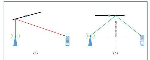
Figure 2: Scenario I (a): In the presence of reconfigurable metasurfaces, the angle of incidence and reflection are not necessarily the same. Scenario II (b): According to Snell's law of reflection, the angle of incidence and reflection are the same.
