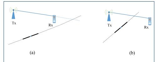
Figure 3: Illustration of Event 1 based on Approach 1. (a) Event 1 holds true if the intersection point between the infinite lines falls outside the Tx-Rx line segment. (b) Otherwise, Event 1 does not hold true.
