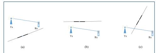
Figure 4: Illustration of Event 1 based on Approach 2. Event 1 holds true if both Tx and Rx are above (a) or below (b) the infinite line corresponding to the typical object. Event 1 does not hold true if Tx and Rx are not on the same side of the line (c).
