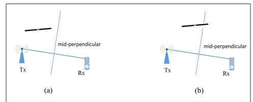
Figure 5: Illustration of Event 3. In (a), Event 1 and Event 2 hold true: The typical object acts as a reflector. In (b), Event 1 holds true but Event 2 does not hold true: The typical object cannot be a reflector.
