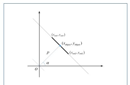
Figure 6: Geometric representation of the typical object in polar coordinates.
