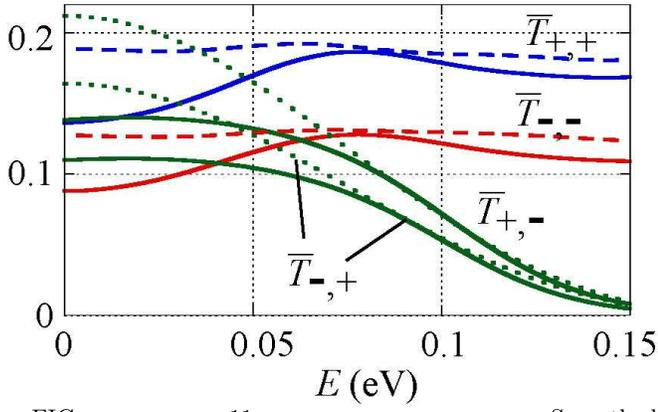
FIG. 11. Smoothed transmission rates  $\frac{1}{3} \sum_{j=-1}^1 T_{\sigma',\sigma}(N+j)$  as a function of the energy  $E$  for the junction of Fig. 5 when  $N = 82$ . Solid and dashed lines represent the exact results and the approximate formulas, respectively.
