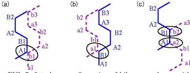
FIG. 7. Interlayer configuration of bilayer graphenes with (a) Ab, (b) Ba and (c) Aa stacking. Here (A,B) and (a,b) denote sublattices in lower  $\downarrow$  and upper  $\uparrow$  layers, respectively.
