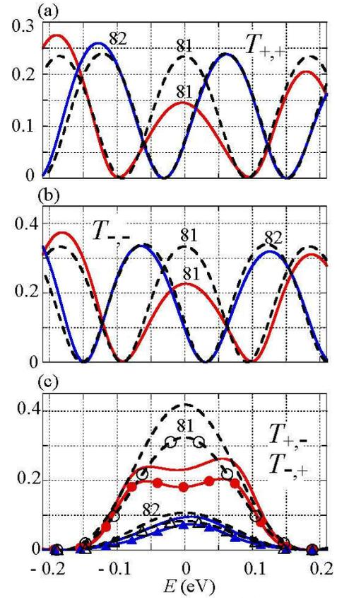
FIG. 9. Transmission rates (a)  $T_{+,+}$  (b)  $T_{-,-}$  and (c)  $T_{\pm,\mp}$  of the junction of Fig. 5 as a function energy  $E$  when  $N = 81, 82$ . Solid and dashed lines represent the exact results and the approximate formulas, respectively. In (c), solid lines with closed symbols and dashed lines with open symbols correspond to  $T_{-,+}$ .
