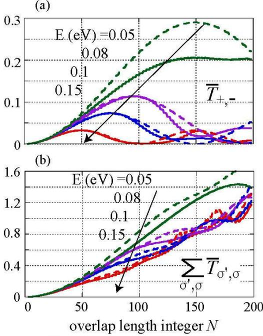
FIG. 8. (a)  $\bar{T}_{+,-}$  and (b)  $\sum_{\sigma'=\pm} \sum_{\sigma=\pm} \bar{T}_{\sigma',\sigma}$  for the energies  $E = 0.05, 0.08, 0.1$  and  $0.15$  eV. Solid and dashed lines represent the exact results and the approximate formulas, respectively. Here  $\bar{T}_{\sigma',\sigma}(N)$  denotes the smoothed transmission rate of the junction of Fig. 5 defined by  $\frac{1}{3} \sum_{j=-1}^1 T_{\sigma',\sigma}(N+j)$ .
