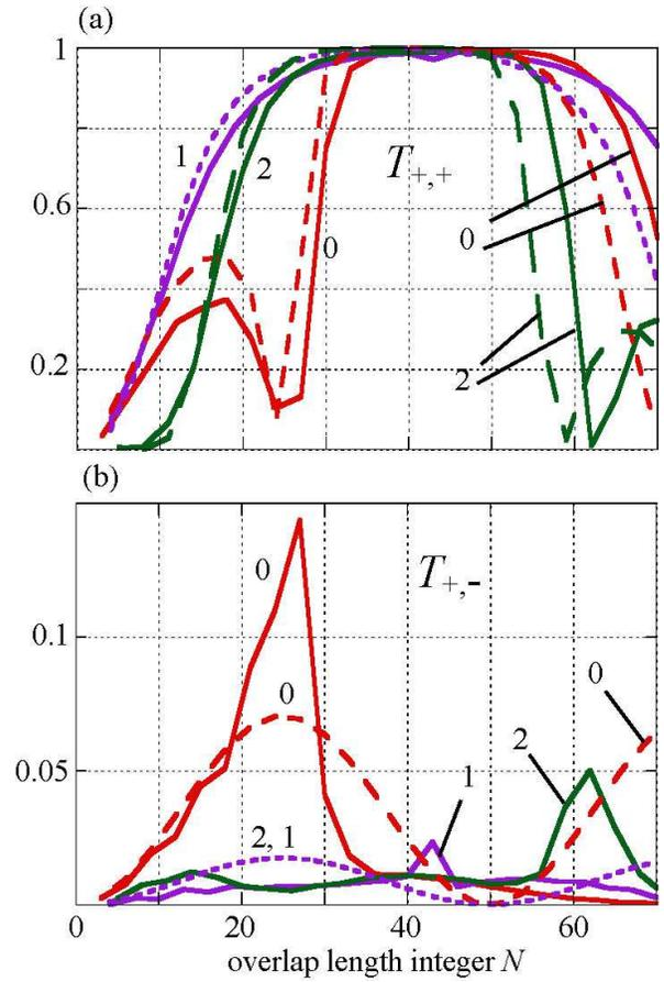
FIG. 6. Transmission rates (a)  $T_{+,+}$  and (b)  $T_{+,-}$  of the coaxial contact  $(n_{\downarrow}, n_{\uparrow}) = (10, 15)$ ,  $j_l = -1$ ,  $\Delta\theta = 0$ ,  $\Delta z = 0$  with the energy  $E = 0.30$  eV. The horizontal axis is the integer  $N$ . Solid and dashed lines represent the exact results and the approximate formulas, respectively. The attached integers 0, 1 and 2 represent mod( $N, 3$ ).
