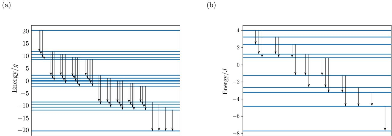
FIG. S1. Possible paths via which an excitation can be cooled down to the ground state. Each black arrow corresponds to an energy difference  $\Delta - \gamma \leq E_i - E_j \leq \Delta + \gamma$ . Each cooling step leads to a reduction of the energy of the system, eventually reaching the ground state. The energy levels are shown for (a) the Ising model ( $N = 5$ ,  $J/g = 5$ ,  $\gamma/g = 3.5$ ) and (b) the Heisenberg model ( $N = 5$ ,  $\gamma/J = 1.26$ ).
