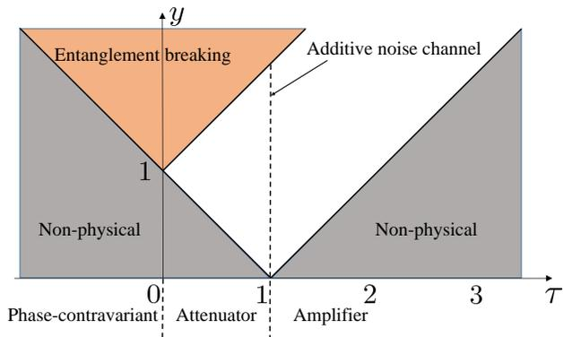
FIG. 1: (Color online) Classification of phase-insensitive single-mode Gaussian channels. Axes defined by  $\tau = \det X$ ,  $y = \sqrt{\det Y}$ . Physical channels (CPTP) should satisfy the relation  $y \geq |\tau - 1|$ . EB channels are on the (orange online) region of  $y \geq |\tau| + 1$ .
